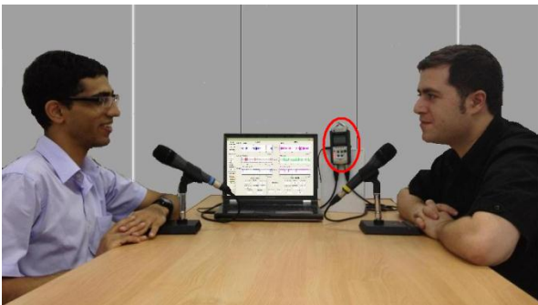
Figure 6: Recording setup using the Zoom H4n voice recorder (circled in red) with Sennheiser e845s microphones for two people conversation.
