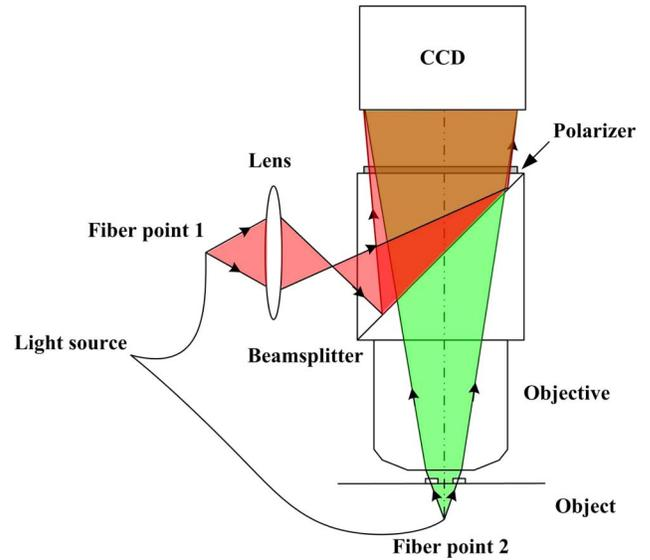
Fig. 4. (Color online) Schematic of transmission-mode DHM setup.
