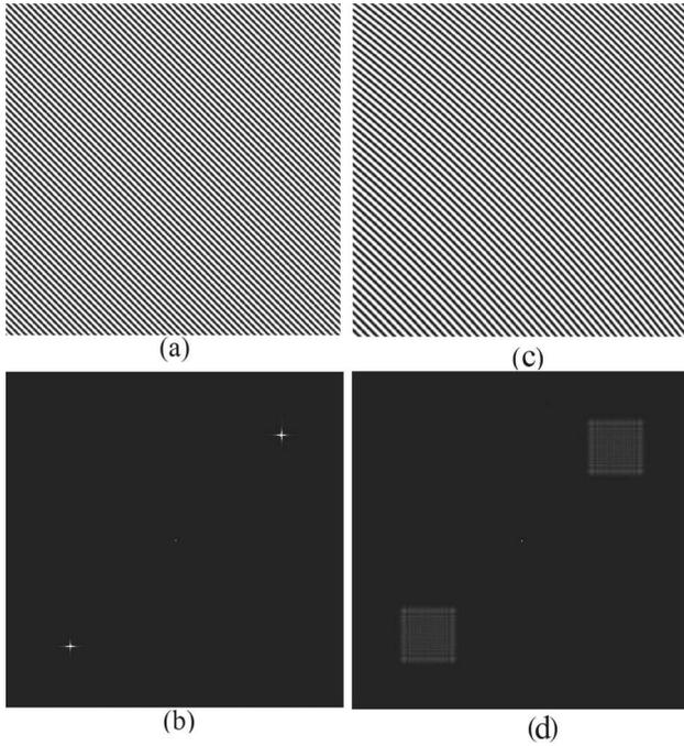
Fig. 2. Spectrum analysis of holograms with different fringe patterns. (a) Hologram with straight fringe pattern. (b) Fourier spectra of hologram (a). (c) Hologram with circular fringe pattern. (d) Fourier spectra of hologram (c).
