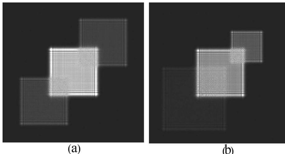
Fig. 7. Fourier spectra of holograms when the numerical spherical reference wave is used to illuminate the holograms. (a) Fourier spectra of the hologram in Fig. 2(a). (b) Fourier spectra of the hologram in Fig. 2(c).
