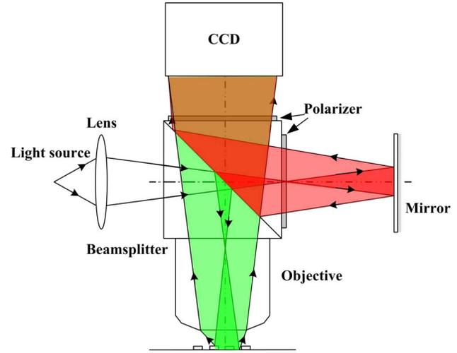
Fig. 3. (Color online) Schematic of the reflection-mode DHM setup.
