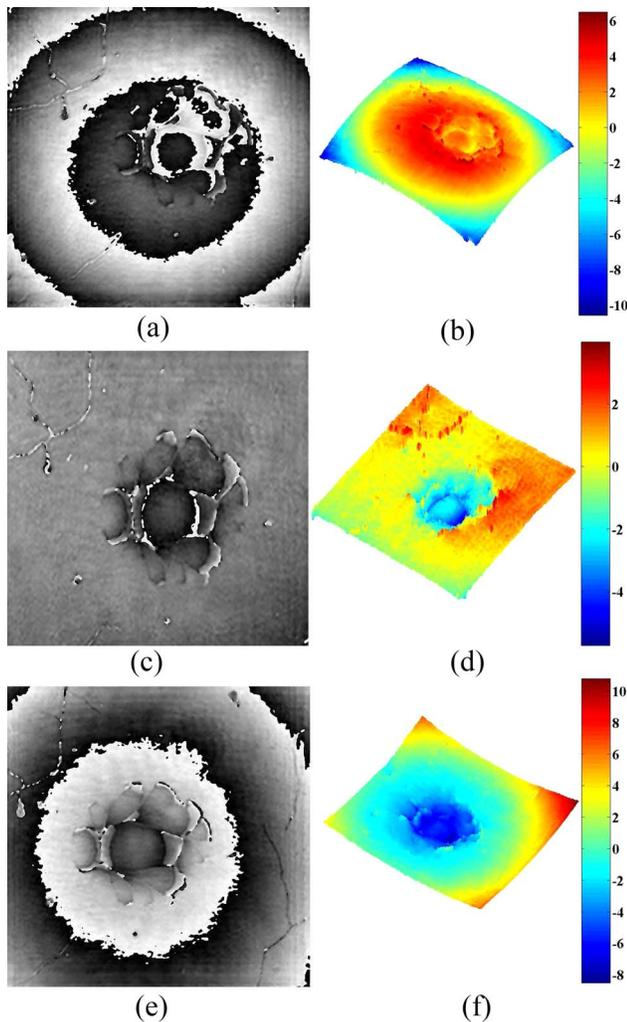
Fig. 6. (Color online) Physical phase compensation demonstration. (a) when  $h_o > h_r$ , a diverging spherical phase remains. (b) Unwrapped 3D phase map of (a). (c) when  $h_o = h_r$ , the spherical phase is totally compensated. (d) Unwrapped 3D phase map of (c). (e) when  $h_o < h_r$ , a converging spherical phase remains. (f) Unwrapped 3D phase map of (e).
