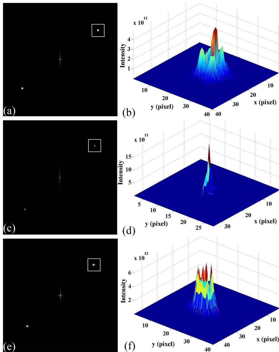
Fig. 5. (Color online) Fourier spectra in the frequency domain. (a) When  $h_o > h_r$ , Fourier spectra of the recording hologram. (b) Spectrum of the plus order with rectangular shape. (c) Fourier spectra of the recording hologram when  $h_o = h_r$ . (d) Spectrum of the plus order with point shape. (e) Fourier spectra of the recording hologram when  $h_o < h_r$ . (f) Spectrum of the plus order with rectangular shape.
