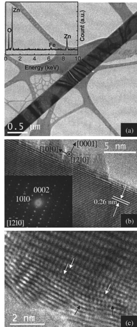
FIG. 3. (a) Low magnification TEM image of a nanobelt inserted with the EDX spectrum; (b) a high resolution TEM image of the nanobelt edge with SAED pattern inserted; and (c) a high resolution TEM image of a nanobelt edge. The white and black arrows in (c) mark the stacking faults and the bending of lattice fringes, respectively.
