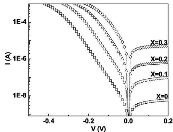
**Figure 6.** Current-voltage characteristics of TiN/Ti capped  $\text{Er}(\text{Si}_{1-x}\text{Ge}_x)_{2-y}$  diodes ( $x = 0-0.3$ ) measured at  $25^\circ\text{C}$ .
