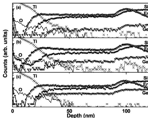
**Figure 5.** SIMS depth profile of  $\text{Er}(\text{Si}_{1-x}\text{Ge}_x)_{2-y}/\text{Si}_{1-x}\text{Ge}_x(100)$  samples after RTA  $600^\circ\text{C}/60$  s in  $\text{N}_2$  ambient using an ION-TOF SIMS with a Ga ion beam. (a)  $x = 0.1$ , (b)  $x = 0.2$ , and (c)  $x = 0.3$ .
