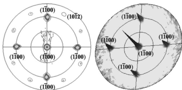
**Figure 2.** Two and three dimensional pole figure XRD scan of  $\text{Er}(\text{Si}_{0.8}\text{Ge}_{0.2})_{2-y}/\text{Si}_{0.8}\text{Ge}_{0.2}(100)$  centered at the  $\text{Er}(\text{Si}_{1-x}\text{Ge}_x)_{2-y}(1\bar{1}00)$   $2\theta$  peak at  $27^\circ$ .
