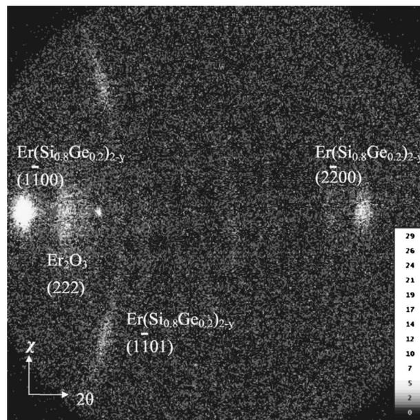
Figure 1. X-ray diffraction GADDS (general area detector diffraction system) scan of  $\text{Er}(\text{Si}_{0.8}\text{Ge}_{0.2})_{2-y}/\text{Si}_{0.8}\text{Ge}_{0.2}(100)$  samples after RTA 600°C/60 s.
