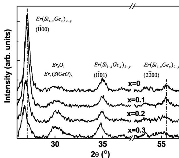
**Figure 3.** X-ray diffraction single crystal  $\theta$ - $2\theta$  plots of  $\text{Er}(\text{Si}_{1-x}\text{Ge}_x)_{2-y}$  samples with varying Ge concentrations. Dotted lines indicate the positions of the  $\text{Er}(\text{Si}_{1-x}\text{Ge}_x)_{2-y}(1\bar{1}00)$  and  $(2\bar{2}00)$  ( $x = 0$ ) peaks, respectively.
