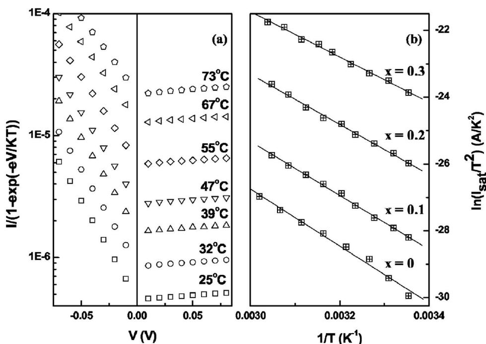
Figure 7. (a) Temperature dependent  $\log(I/(1 - \exp[-(eV/kT)]))$   $I$ - $V$  plots measured on  $\text{Er}(\text{Si}_{1-x}\text{Ge}_x)_{2-y}$  diodes ( $x = 0.2$ ) with typically low leakage currents. (b) Richardson's plot for  $\text{Er}(\text{Si}_{1-x}\text{Ge}_x)_{2-y}$  diodes ( $x = 0-0.3$ ).
