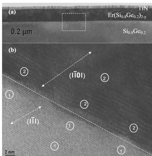
**Figure 4.** XTEM micrographs of the  $\text{Er}(\text{Si}_{0.8}\text{Ge}_{0.2})_{2-y}/\text{Si}_{0.8}\text{Ge}_{0.2}(100)$  interface. (a) The top XTEM micrograph shows the germanosilicide/SiGe interface at low magnification. (b) The bottom XTEM micrograph shows the bright field HRTEM of the interface indicated by the dotted white box in (a). TEM/EDX analysis was done on the circled regions.
