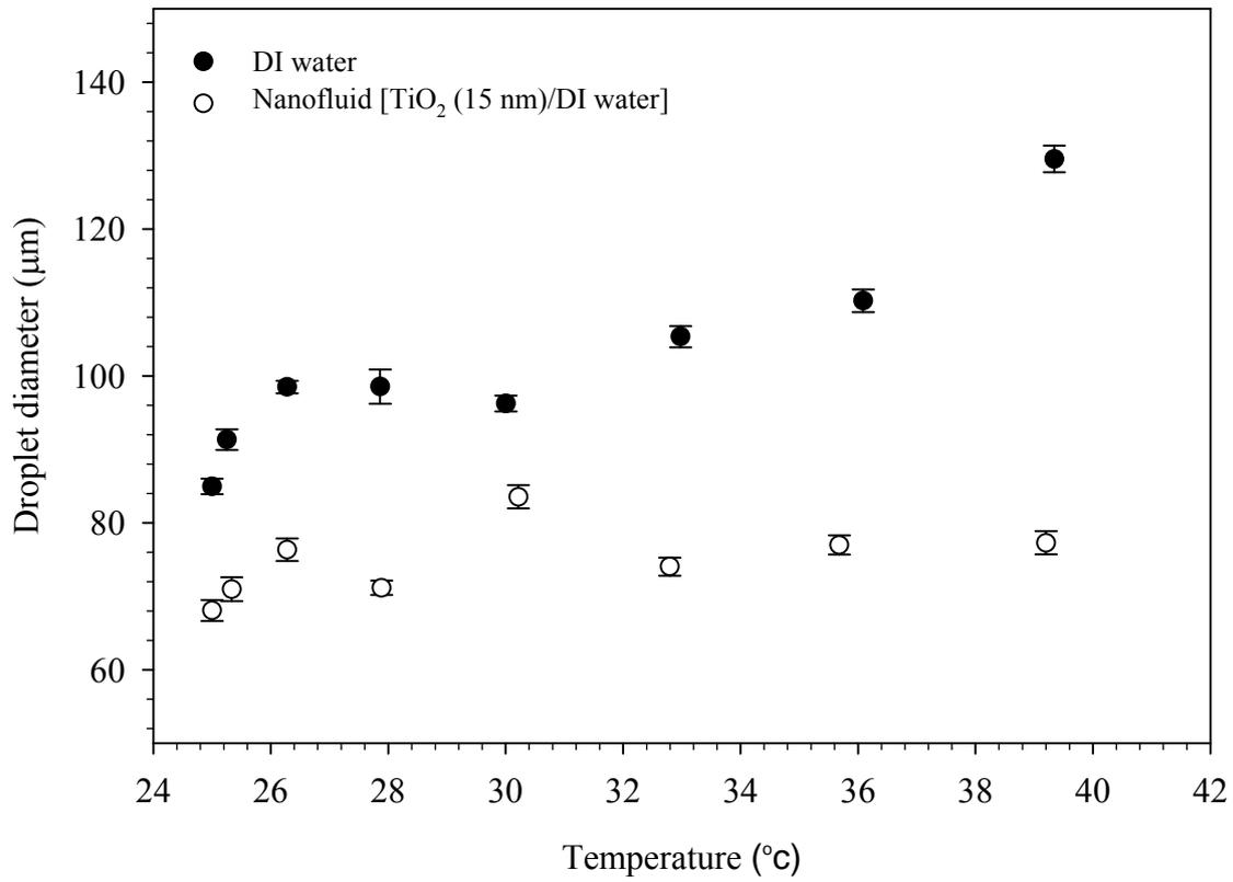
**Fig. 6** Temperature dependence of droplets size of DI water and a nanofluid at 30 μm depth microchannel (Both DI water and nanofluid had same flow rates of 6 μl/h and oil flow rate was 12 μl/h)
