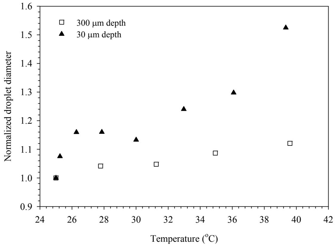
**Fig. 4** Effect of microchannels depths on DI water droplet size at a constant flow rate ratio (DI water/oil) of 1:2 and average flow velocity (Droplet diameters are normalized by their nominal values at 25°C. At 25°C, the droplet sizes formed in the T-junctions of 300 μm and 30 μm channel depths are 334 μm and 85 μm, respectively.)
