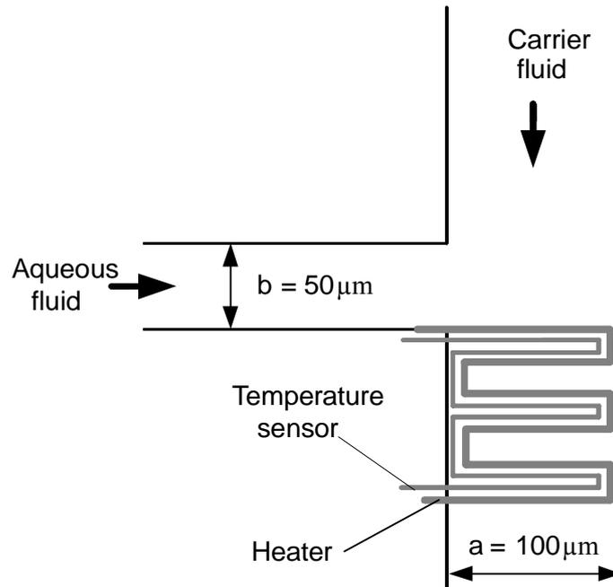
**Fig. 1** Schematic concept of a T-junction with integrated microheater and temperature sensor
