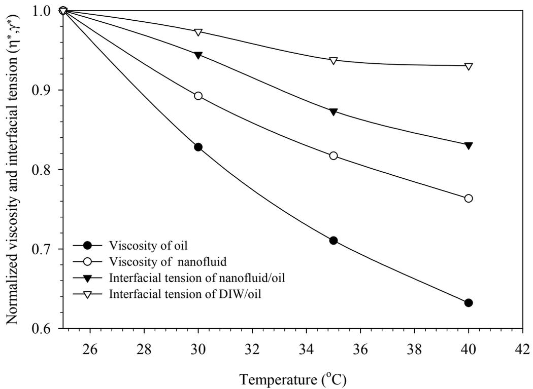
**Fig. 2** Temperature-dependent viscosity and interfacial tension of the investigated fluids (Viscosities and interfacial tensions are normalized by their nominal values at 25°C. At 25°C, viscosities of mineral oil and nanofluid are 26.4 mPa.s and 0.93 mPa.s, respectively, the interfacial tension of DIW/oil and nanofluid/oil systems are 27.35 mN/m and 15.9 mN/m, respectively)
