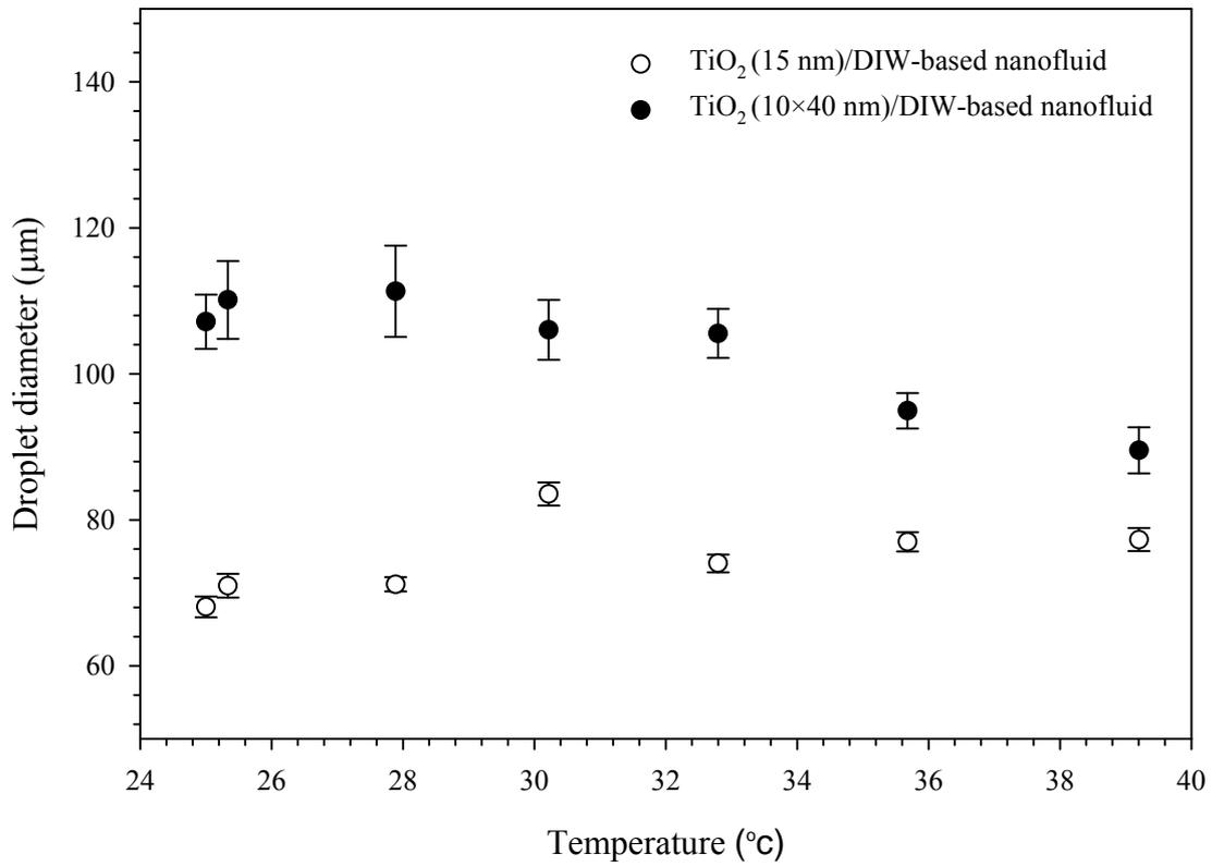
**Fig. 7** Effect of nanoparticle shape on temperature-dependent droplet size formed in T-junction of 30 μm channel depth at constant flow rates of 6 μl/h and 12 μl/h for nanofluids and oil, respectively
