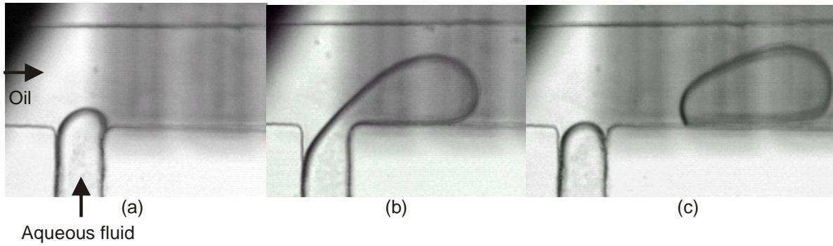
**Fig. 3** Deionized water droplet formation at 30  $\mu\text{m}$  channel depth T-junction (Water and oil flow rates are 6  $\mu\text{l/h}$  and 12  $\mu\text{l/h}$ , respectively): (a) forming; (b) before detachment; (c) droplet after detachment
