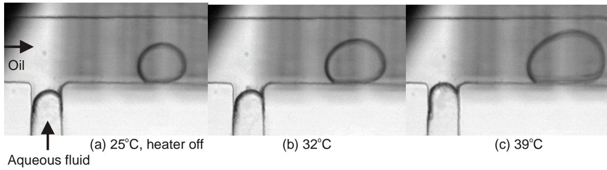
**Fig. 5** Variation of DI water droplet size at different temperatures at 30  $\mu\text{m}$  depth microchannel (flow rates of 6  $\mu\text{l/h}$  for water and 12  $\mu\text{l/h}$  for oil): (a) 25°C; (b) 32°C, (c) 39°C
