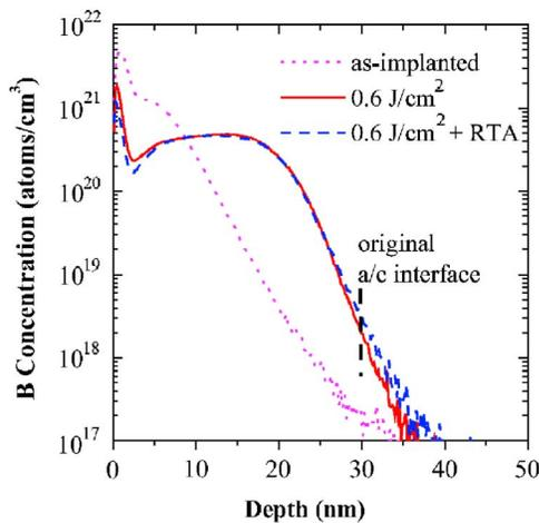
FIG. 1. (Color online) SIMS profiles of boron subjected to LA at  $0.6 \text{ J/cm}^2$  with or without a post-LA low temperature RTA at  $600^\circ\text{C}$  for 60 s. Minimum diffusion near the tail region occurred due to the additional RTA cycle. The  $\text{B}^+$  implantation was performed at 0.5 keV with a dose of  $1 \times 10^{15} \text{ cm}^{-2}$ , while the  $\text{Si}^+$  amorphization implantation was conducted at 10 keV with a dose of  $2 \times 10^{15} \text{ cm}^{-2}$ .
