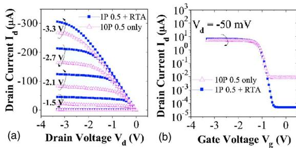
FIG. 4. (Color online) (a) Drain current ( $I_d$ ) vs drain bias ( $V_{ds}$ ) and (b) drain current ( $I_d$ ) vs gate bias ( $V_{gs}$ ) characteristics of a  $0.5 \mu\text{m}$   $p$ -MOSFET subjected to a single-pulse LA at  $0.5 \text{ J/cm}^2$  with a post-LA RTA at  $600^\circ\text{C}$  for 60 s or only to a ten-pulse LA at  $0.5 \text{ J/cm}^2$ . The low drive current is due to unsilicided source/drain and gate regions. The implantation conditions are the same as those used in Fig. 2.
