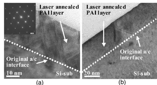
FIG. 3. Cross-sectional transmission electron microscopy micrographs of unpatterned PAI samples subjected to a single-pulse LA at (a)  $0.5 \text{ J/cm}^2$  only and (b)  $0.5 \text{ J/cm}^2$  with a post-LA RTA at  $600^\circ\text{C}$  for 60 s. The inset in (a) is the electron diffraction pattern showing epitaxial silicon (001) obtained from the recrystallized region that contains crystalline defects. The implantation conditions are the same as those used in Fig. 1.
