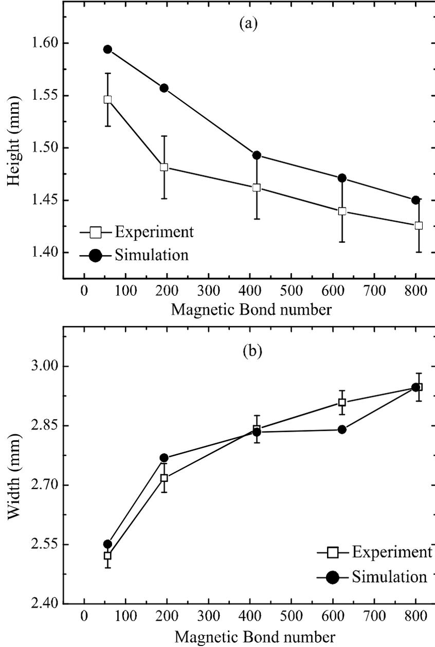
Figure 12: Geometrical parameters as functions of magnetic Bond number of a 4.8- $\mu\text{L}$  ferrofluid droplet: (a) height; (b) width.
