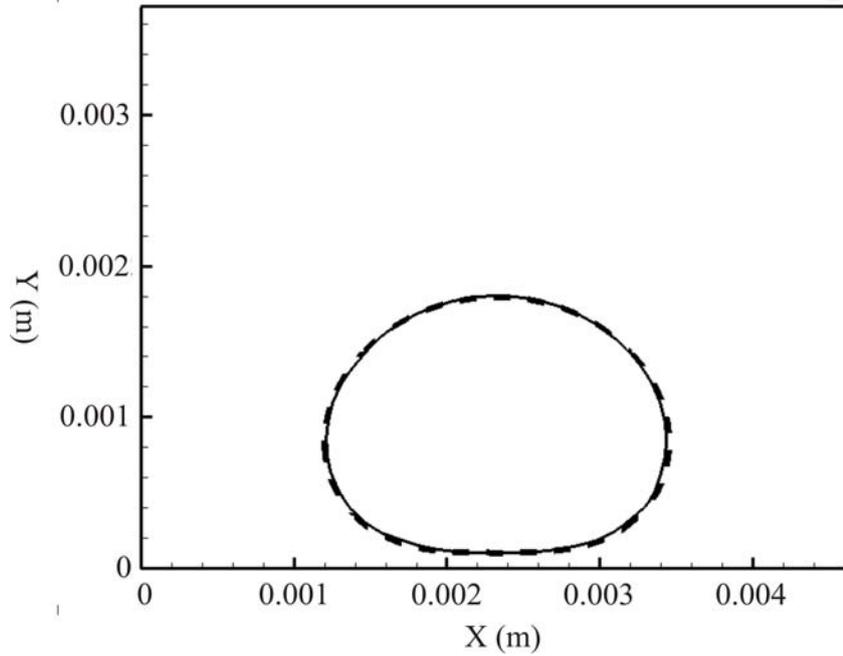
Figure 8: Grid-independent study with droplet in the computational domain (solid line:  $42 \times 34 \times 26$  CVs at a time step of  $\Delta t = 1 \times 10^{-3} s$ , dashed line:  $62 \times 50 \times 38$  CVs at a time step of  $\Delta t = 5 \times 10^{-4} s$ ).
