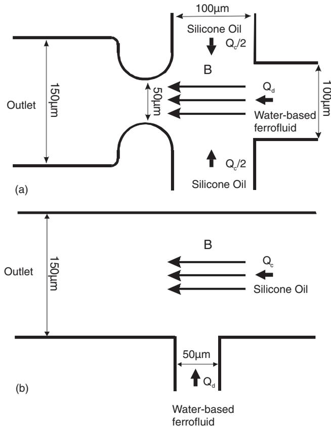
FIG. 1. Schematic of the microfluidic geometries used (not drawn to scale): (a) flow-focusing and (b) T-junction configurations. In the flow-focusing configuration, the magnetic field is aligned parallel to the dispersed phase fluid. In the T-junction configuration, the magnetic field is aligned perpendicular to the dispersed phase fluid.
