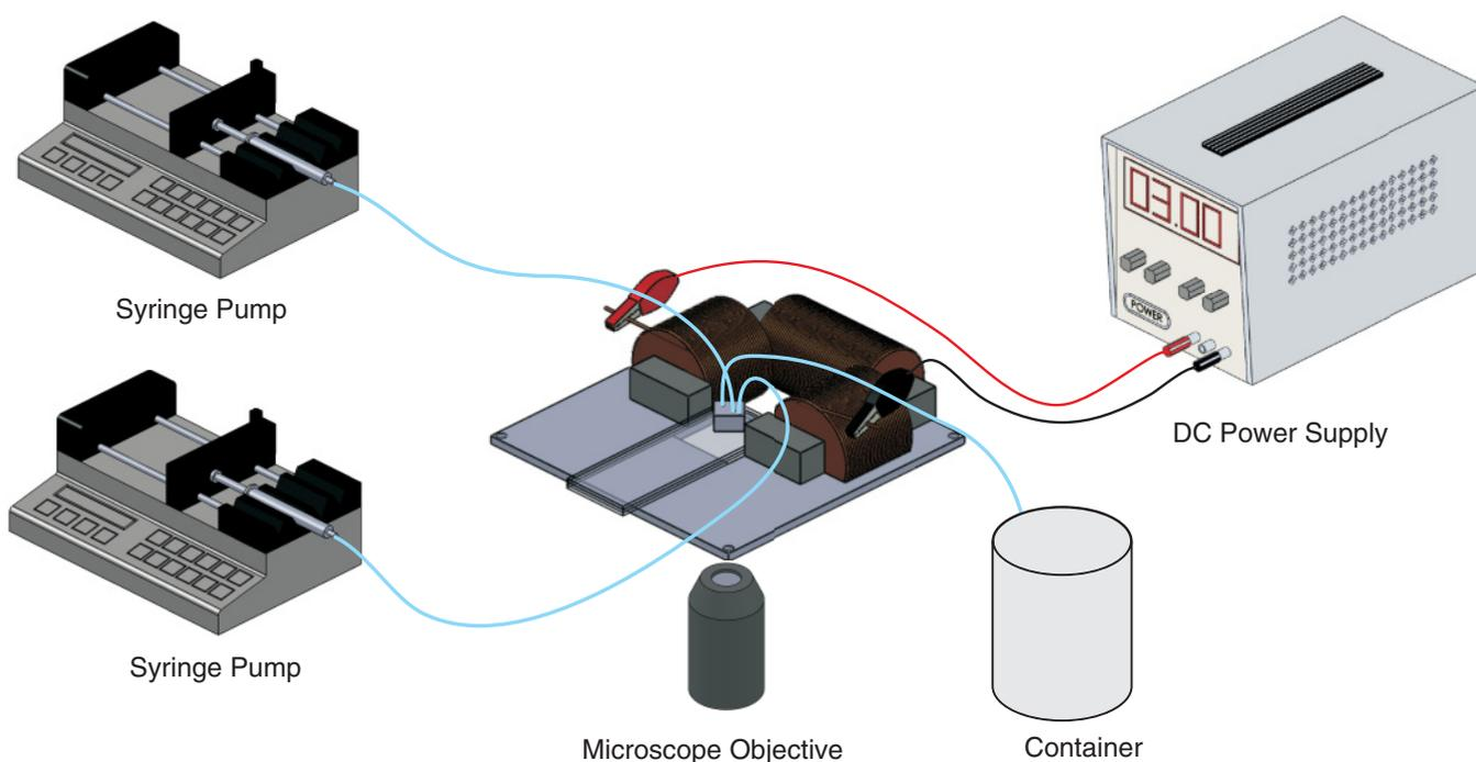
FIG. 3. (Color online) Schematic of the experimental setup (not drawn to scale): (a) top view and details of the electromagnet and (b) experimental setup.
