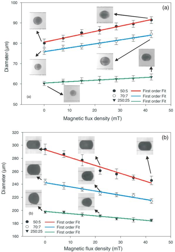
FIG. 5. (Color online) Size of ferrofluid emulsions as a function of magnetic flux density: (a) flow-focusing configuration and (b) T-junction configuration. Each symbol represents the flow rates of the CP:DP in  $\mu\text{l h}^{-1}$ . Each colored line represents different fixed flow rates.
