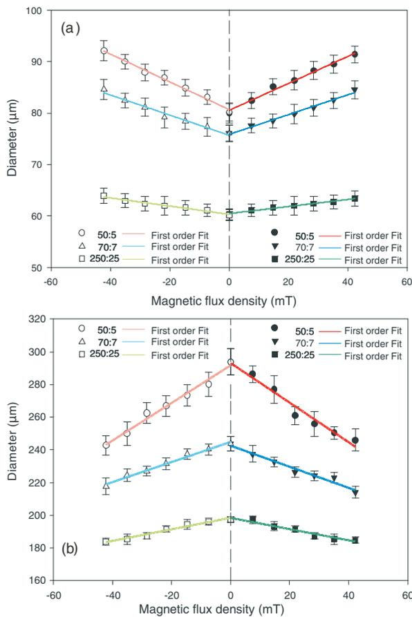
FIG. 8. (Color online) Effect of the polarity of the magnetic field. Each colored line represents different fixed flow rates used. The dark colored lines represent the ferrofluid emulsions formed using a positive magnetic flux density. The light colored lines represent the ferrofluid emulsion formed using a negative magnetic flux density. Each symbol represents the flow rates used in  $\mu\text{l h}^{-1}$  (a) using the flow-focusing geometry and (b) using the T-junction geometry.
