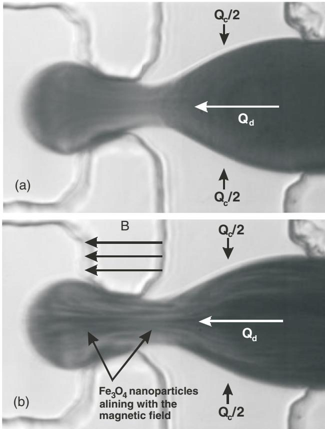
FIG. 6. Alignments of the clustered magnetic nanoparticles in the direction of the magnetic field. In both cases, the flow rates are fixed at 50:5 (CP:DP in  $\mu\text{l h}^{-1}$ ): (a) without magnetic field and (b) at magnetic flux density of 42.3 mT.
