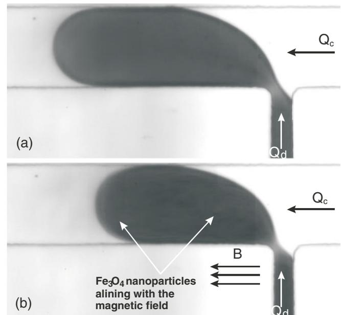
FIG. 7. Alignment of the clustered magnetic nanoparticles in the direction of the magnetic field. In both cases, the flow rates are fixed at 50:5 (CP:DP in  $\mu\text{l h}^{-1}$ ): (a) without magnetic field and (b) at magnetic flux density of 42.3 mT.
