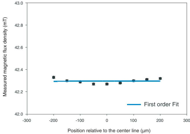
FIG. 4. (Color online) Measured magnetic flux density as a function of position relative to the centerline. The magnetic field is generated using a constant current of 3 A. The centerline represents the midpoint in the dispersed phase channel. A positive distance indicates the upstream and a negative position indicates the downstream position. The position is adjusted using a micropositioner.
