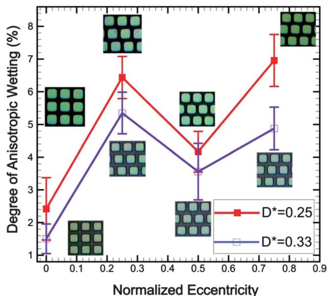
**Fig. 4** Percentage of anisotropic wetting  $\delta$  versus normalized eccentricity  $\epsilon^*$  at different values of relative pillar spacing  $D^*$ .
