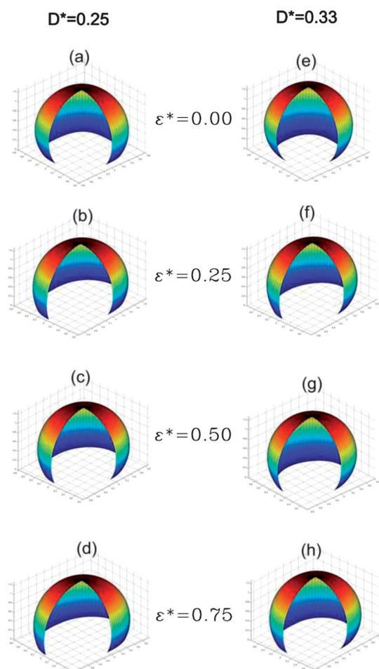
**Fig. 8** Three-quarters of an equilibrium drop shape with  $V = 2 \mu\text{L}$ . From top to bottom, the effects of increasing the pillars eccentricity are shown, *i.e.* (a–d) and (e–h), while from left to right, the effects of increasing the pillars relative spacing are illustrated, *e.g.* (a and e) or (d and h).
