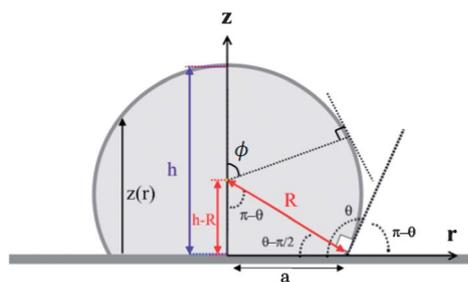
Fig. 7 Axisymmetric drop shape on a hydrophobic surface.
