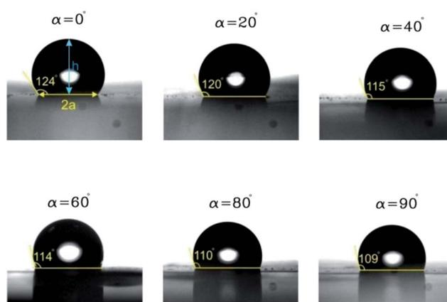
**Fig. 2** Typical images of the contact angle anisotropy of the micropillar surfaces ( $D^* = 0.25$  and  $\varepsilon^* = 0.75$ ) of a single droplet by rotating the sample from (0–90°) in 20° step increments.
