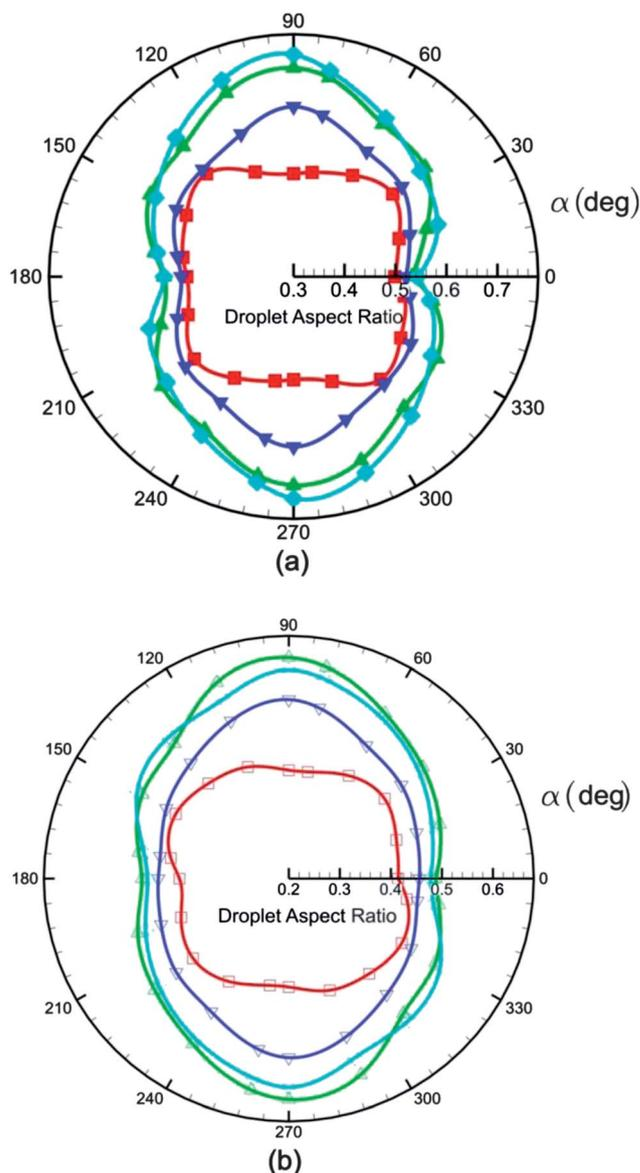
**Fig. 6** Droplet aspect ratio  $a^*$  as a function of viewing angle  $\alpha$  ( $^\circ$ ) on the polar coordinate. Spline interpolation between the experimental data represents the three-phase contact line of the droplet (a)  $D^* = 0.25$ ; (b)  $D^* = 0.33$  (line legend is the same as that of Fig. 3).
