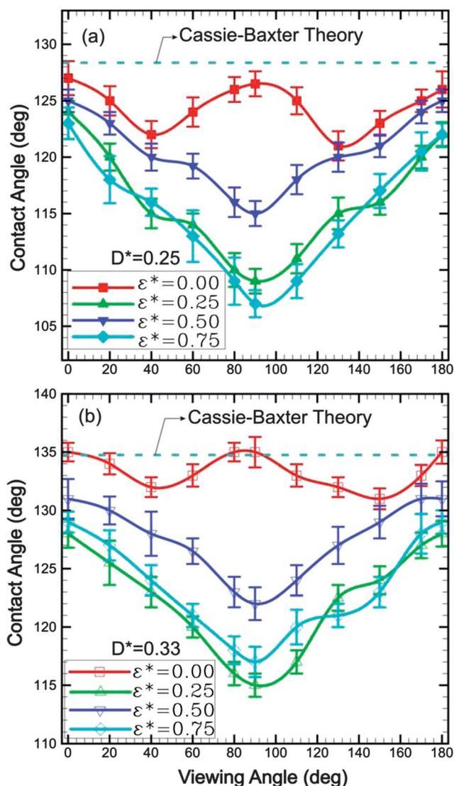
**Fig. 3** Experimental contact angle  $\theta$  versus viewing angle  $\alpha$  at different values of normalized eccentricity  $\epsilon^*$  and relative pillar spacing  $D^*$ . (a)  $D^* = 0.25$ . (b)  $D^* = 0.33$ .
