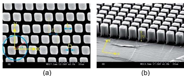
**Fig. 1** Representative SEM images of the fabricated pillars: (a) top view of the micropillars with coordinates and geometrical parameters used in this study. (b) Isometric view of the micropillars,  $\eta = 10 \mu\text{m}$ .
