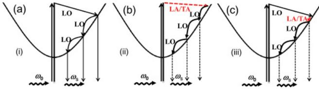
FIG. 6. (Color online) Schematic diagram of acoustic and LO phonon scattering process under resonant condition. (a) Process (i): general multi-LO phonon scattering process. (b) Process (ii): acoustic phonon scattering process followed by LO phonons. (c) Process (iii): LO phonon scattering followed by acoustic phonon.
