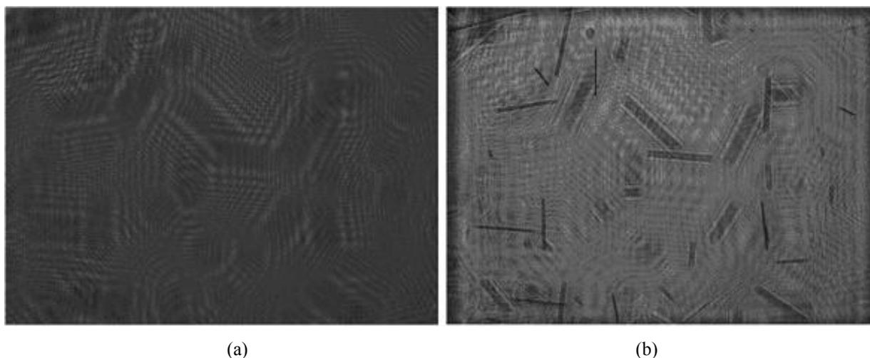
Fig. 5. Digital holographic microscopy data of carbon fiber suspended in water. (a) A recorded digital hologram and (b) Example of a reconstructed image.
