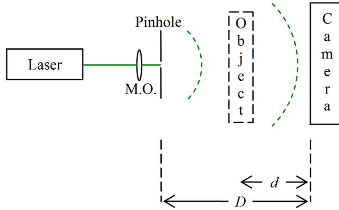
Fig. 2. Digital holographic microscopy setup. M. O. stands for Microscopic Objective lens.
