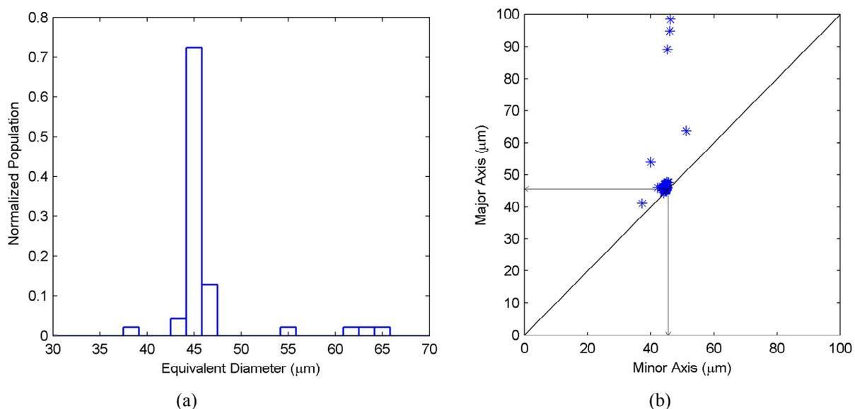
Fig. 8. (a) Particle size distribution of 40  $\mu\text{m}$  polymer microspheres and (b) Axis length distribution of 40  $\mu\text{m}$  polymer microspheres
