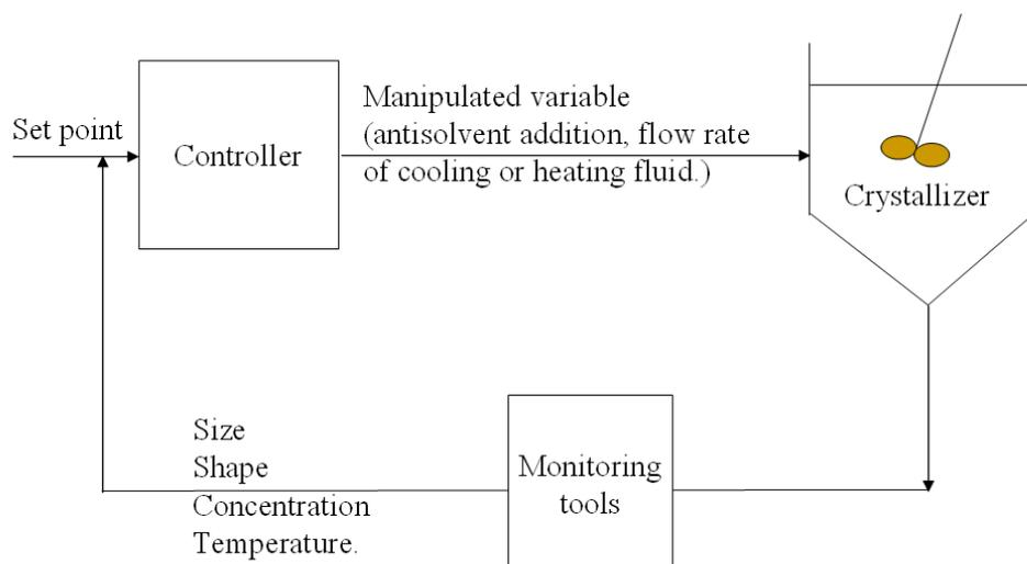
Fig. 1. Feedback control of a crystallizer
