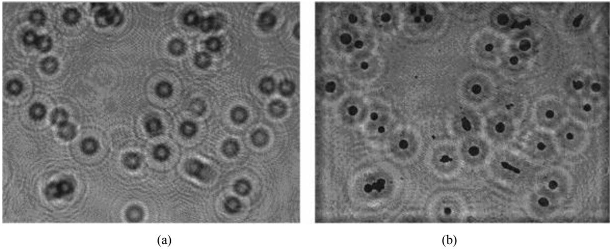
Fig. 3. Digital holographic microscopy data of ceramic beads on glass slide. (a) One of the recorded digital holograms and (b) Example of a reconstructed image
