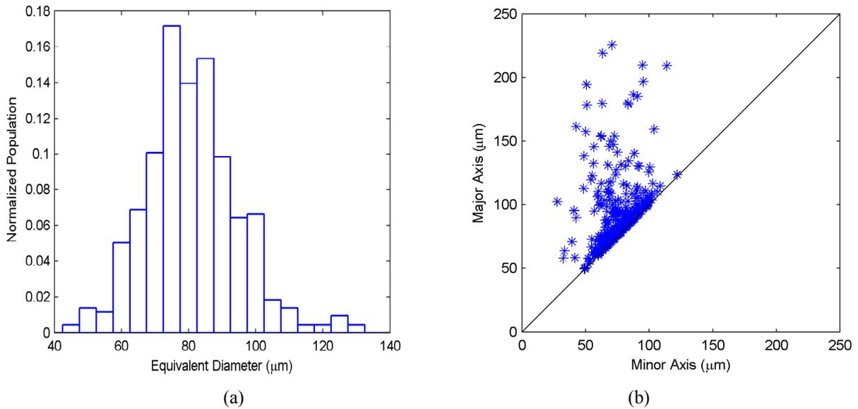
Fig. 4. (a) Particle size distribution of ceramic beads obtained by digital holographic microscopy method. (b) Axis length distribution of spherical ceramic beads. Each asterisk represents the axis length of one particle.
