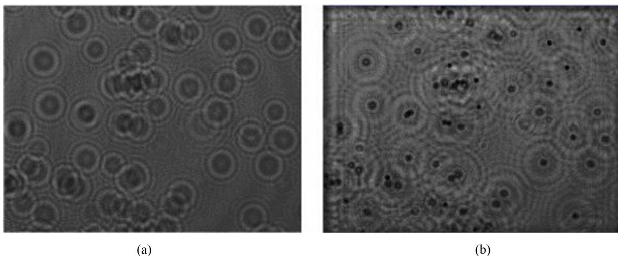
Fig. 7. Digital holographic microscopy data of 40  $\mu\text{m}$  polymer microsphere suspensions through flow cell. (a) A recorded digital hologram and (b) Example of a reconstructed image.
