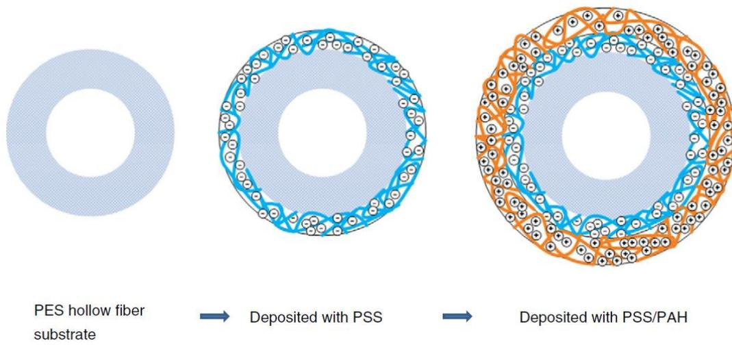
Fig.1. Schematic drawing of layer-by-layer deposition on hollow fiber membrane.
