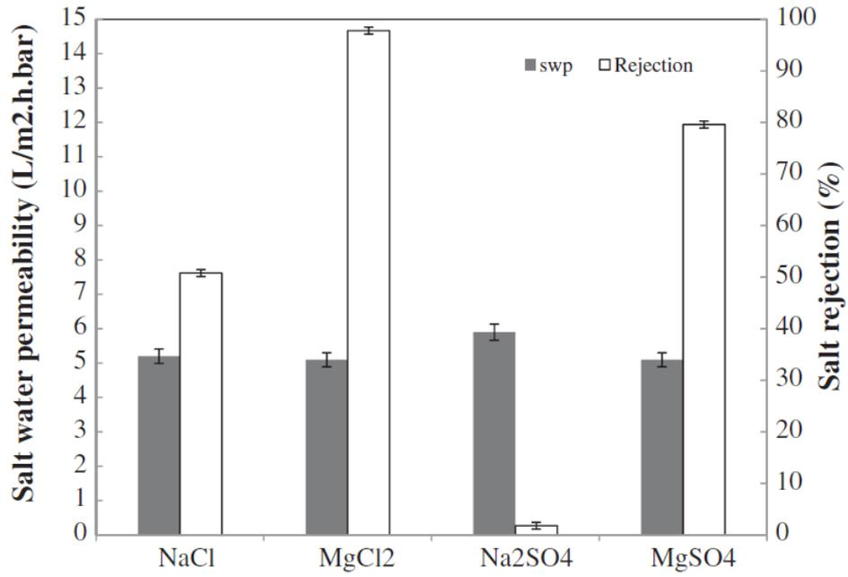
Fig.4. Filtration performances of 6-layer LBL membrane with different salt solutions (tested at 1 bar using 500 ppm salt solution).
