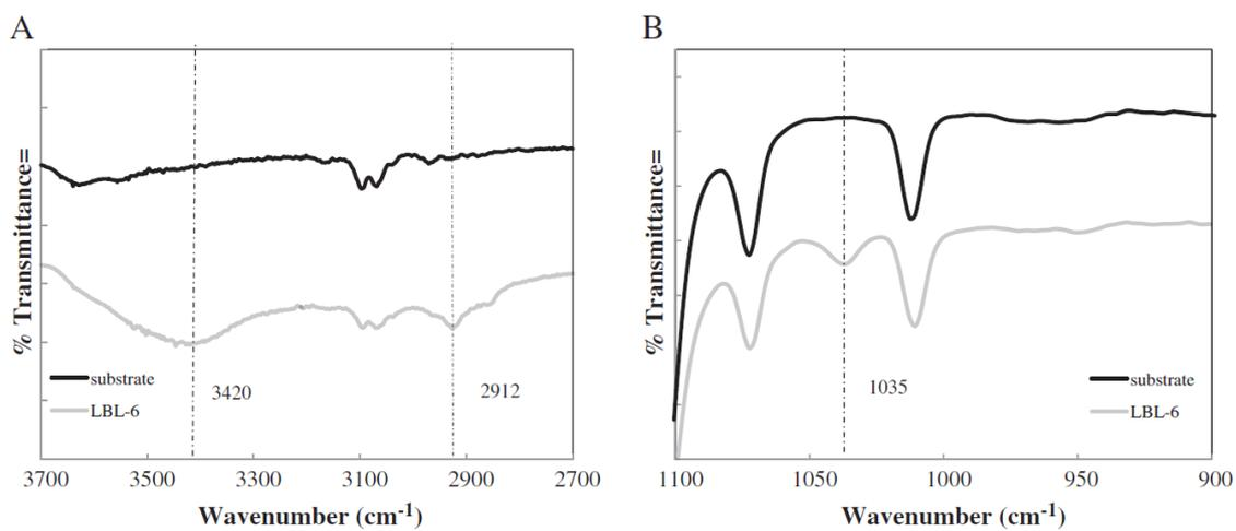
Fig.3. ATR-FTIR spectra of membrane substrate and 6-layer LBL membrane.
