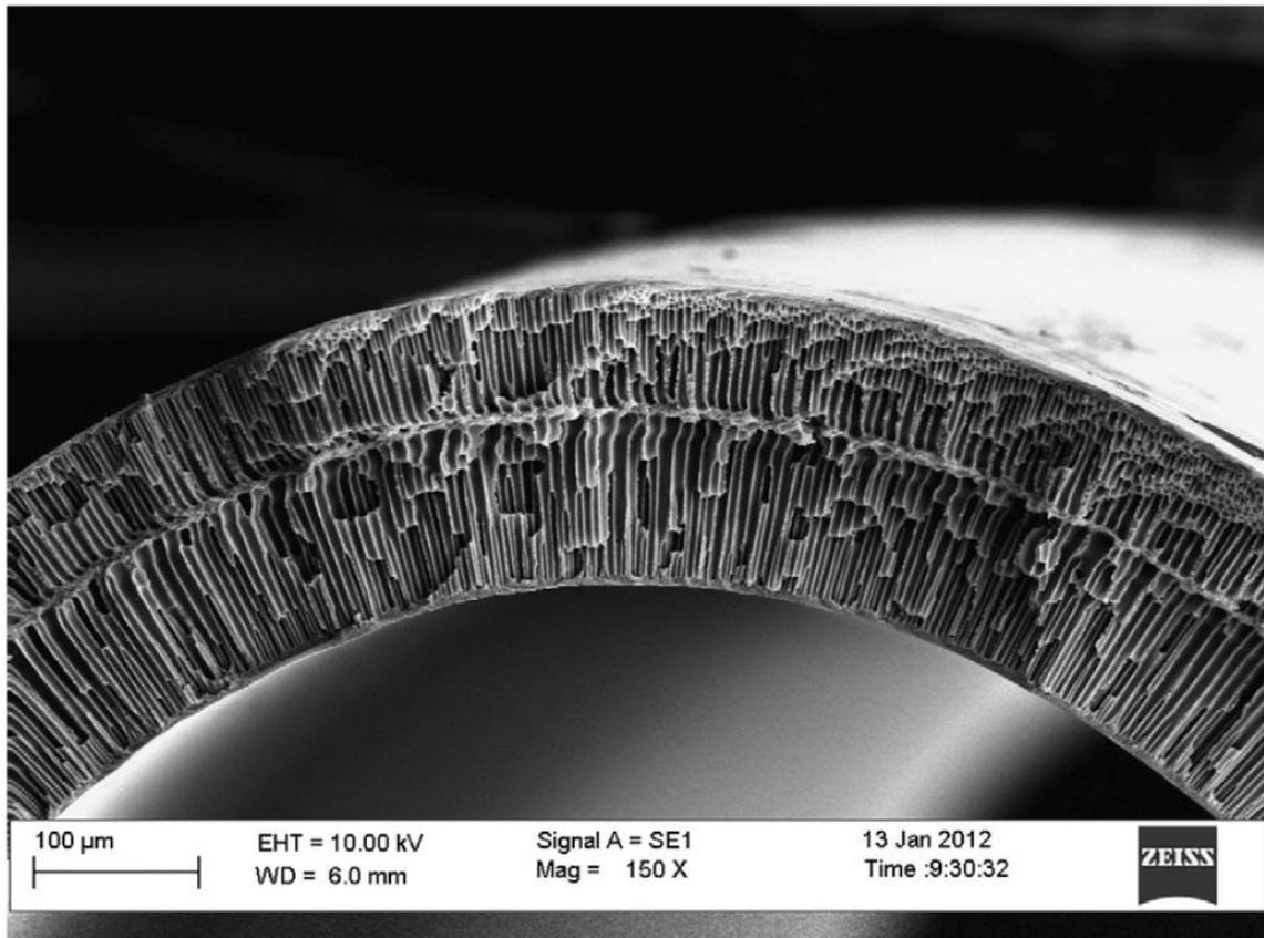
Fig.2. Cross-section morphology of PES hollow fiber substrate at 150x.
