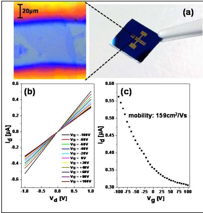
Figure 3: (a) Optical micrograph of the fabricated graphene device. (b) Output characteristics of the transistor device under different applied gate voltages. (c) Current – voltage transfer curve of bottom-gated graphene FET at a drain-source bias of  $V_d = 0.1V$ .
