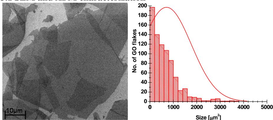
Figure 1: (left) SEM image of a large GO sheet on  $\text{SiO}_2$  substrate produced from the modified method. (right) Size distribution of GO flakes. Solid curve indicates the Gaussian fit.
