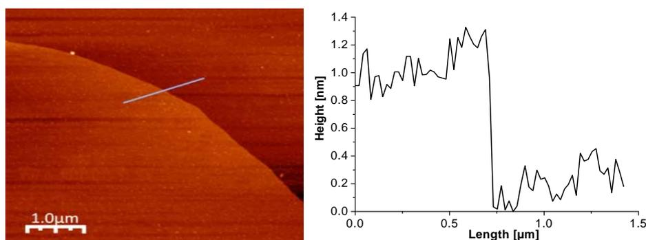
Figure 2: (left) AFM image of GO and (right) AFM height profile for the GO sheet.
