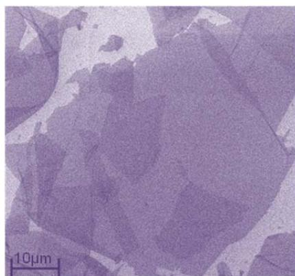
*Figure: SEM image of a large GO sheet on SiO<sub>2</sub> substrate produced from the reported modified method.*
