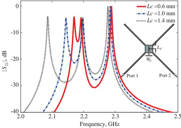
**Figure 3.**  $|S_{21}|$  response under different slot length ( $L_c$ ) ( $W_s=W_c=0.4$  mm,  $L_s=27.2$  mm and  $W_p=3$  mm), with the illustration of the slotted-patch loaded resonator capacitively coupled by  $90^\circ$ -oriented feed lines.
