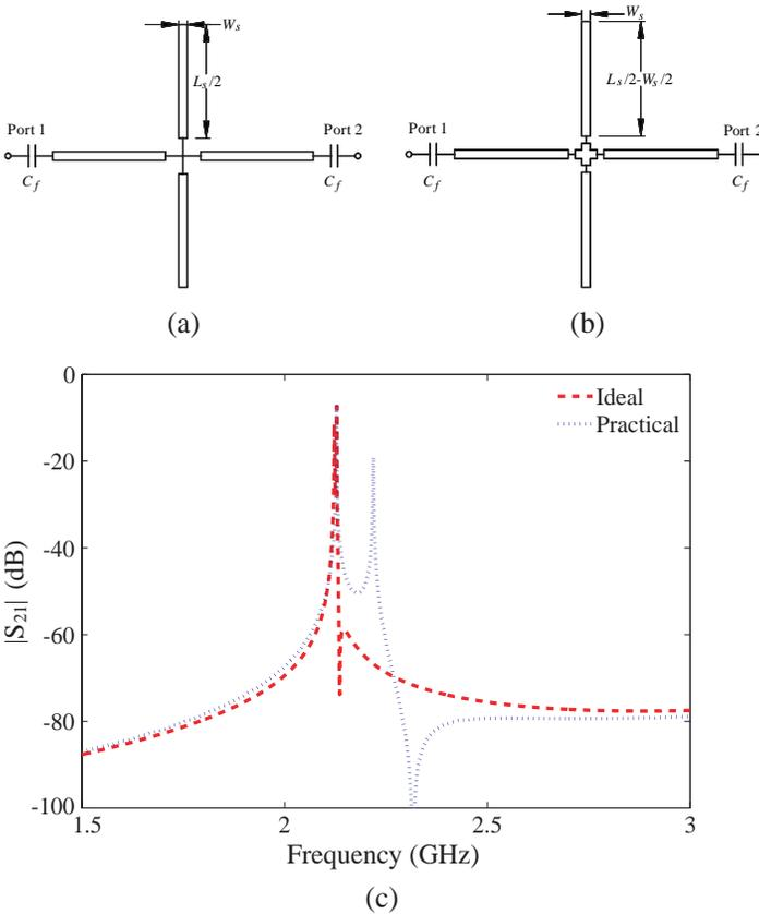
**Figure 1.** The schematic of the cross resonator. (a) Ideal case. (b) Practical case with the cross junction in the center, and for the two cross resonators, they are with the same electric length and under weak coupling condition ( $C_f = 0.001$  pf,  $W_s = 0.4$  mm and  $L_s = 27.2$  mm). (c) Frequency responses for the two cross resonators.
