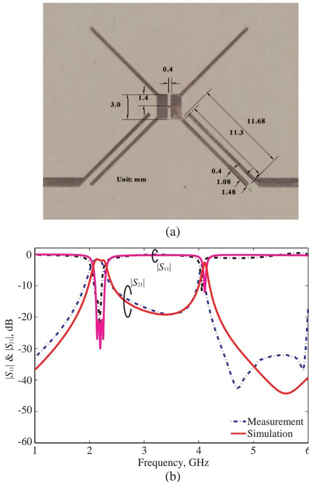
**Figure 4.** (a) Photograph of the fabricated Filter I. (b) Simulated and measured frequency responses of Filter I.
