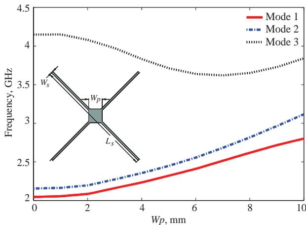
**Figure 2.** Resonant frequencies of the first three modes versus patch size ( $W_p$ ) ( $W_s=0.4$  mm and  $L_s=27.2$  mm), with the illustration of the schematic of the patch loaded cross resonator.
