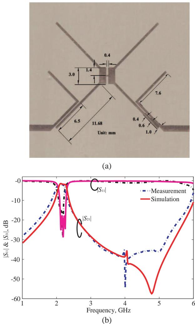
**Figure 5.** (a) Photograph of the fabricated Filter II. (b) Simulated and measured frequency responses of Filter II.
