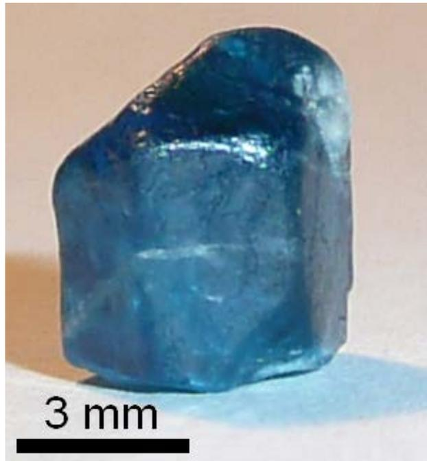
**Figure 2.** The apatite crystal used for the neutron diffraction experiment.
