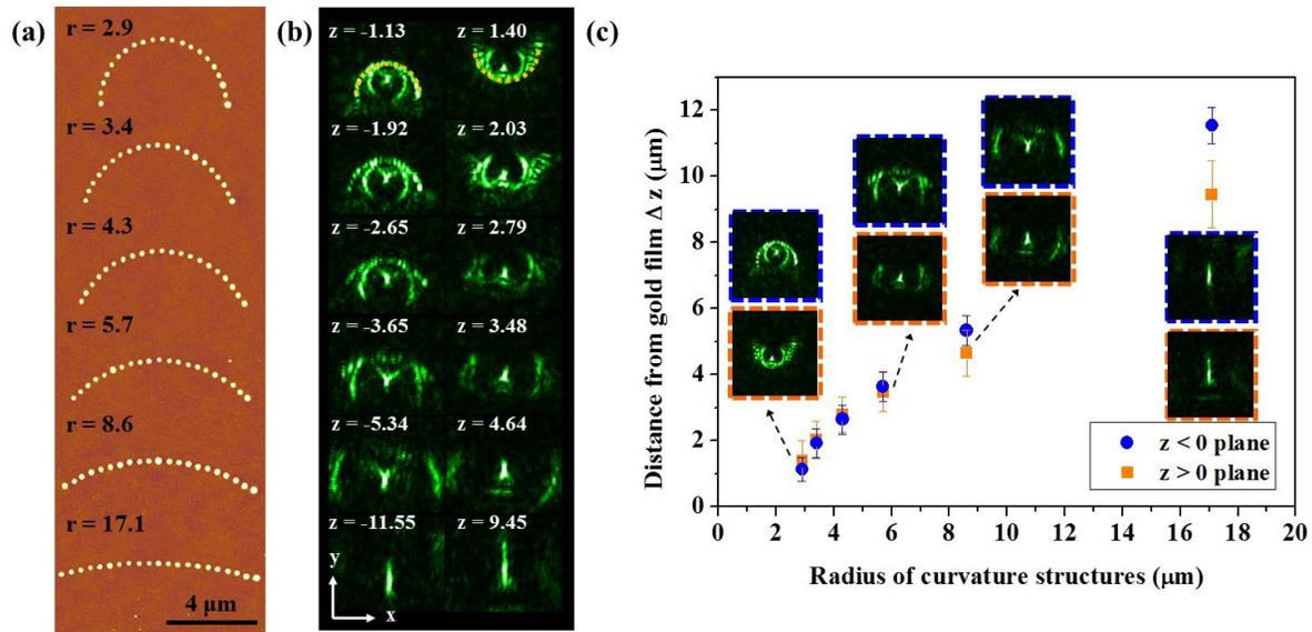
Figure 1. The curve structures with different radii of curvature (RCs). (a) The AFM images of the radii of curvature structure, ranged from  $r = 2.9$  to  $17.1 \mu\text{m}$ . (b) The TIRM optical images of the radii of curvature structure. The left and right columns are the optical images of the concave and convex structure, respectively. (c) The projecting distance from gold film  $\Delta z$  as a function of radii of curvature structures.
