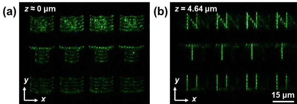
Figure 4. The TIRM images of the designed structure composed of the curved structure. (a) The irregular light pattern in the observation plane  $z \sim 0 \mu\text{m}$ . (b) The clearly optical pattern "NTU" in the designed observation plane,  $z = 4.64 \mu\text{m}$ .
