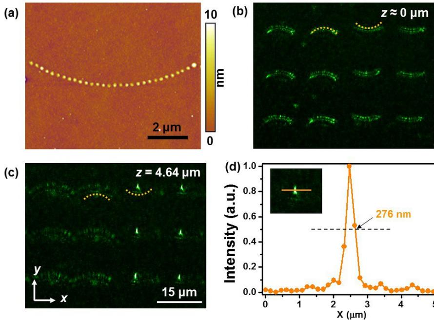
Figure 3. The designed curved structure with  $r = 8.6 \mu\text{m}$  and interspacing of 300 nm. (a) The AFM image of the designed curved structure. (b) The TIRM image observed in the observation plane  $z \sim 0$ . The bright scattering of concave and convex are shown. (c) The TIRM image in the observation plane  $z = 4.64 \mu\text{m}$ . The focusing spot and diverging fringe of convex and concave are observed respectively.
