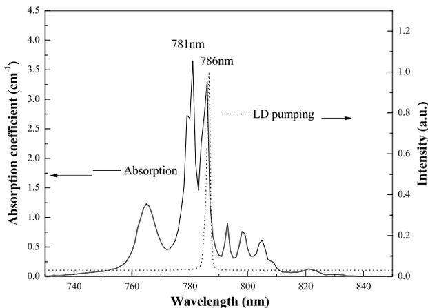
Fig. 2. Absorption spectrum of Tm:YAG ceramic (dotted line) and emission spectrum of LD (solid curve).
