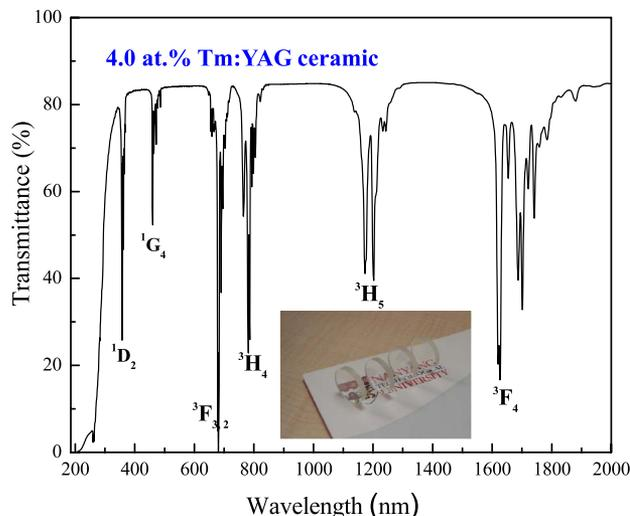
Fig. 1. (Color online) Transmittance spectrum of Tm:YAG ceramic.
