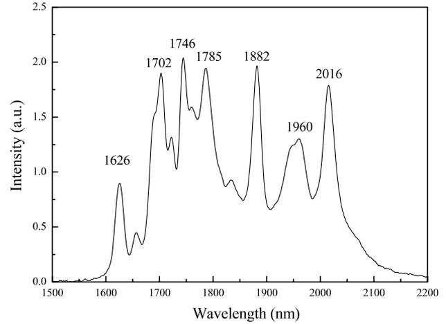
Fig. 3. Fluorescence spectrum of 4 at. % Tm:YAG ceramic.
