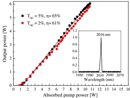
Fig. 5. (Color online) The output power versus absorbed pump power with different output couplings. Inset: the laser spectrum of Tm:YAG ceramic laser.
