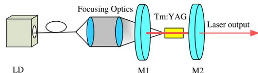
Fig. 4. (Color online) Experimental setup of Tm:YAG ceramic laser.
