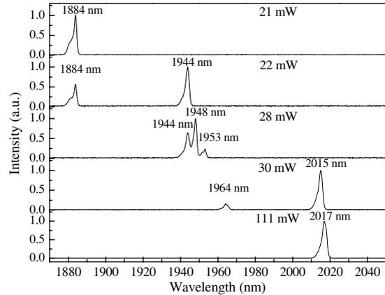
Fig. 6. Wavelength tuning operation of the Tm:YAG ceramic laser.
