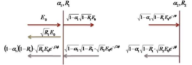
Fig. 4. (Color online) Multiple reflection model of the air bubble.
