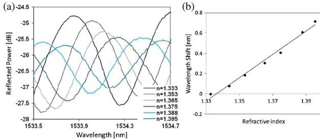
Fig. 7. (Color online) (a) Reflected power for different refractive indices in a wavelength function. (b) Deep position as a function of the refractive index of the surrounding medium.
