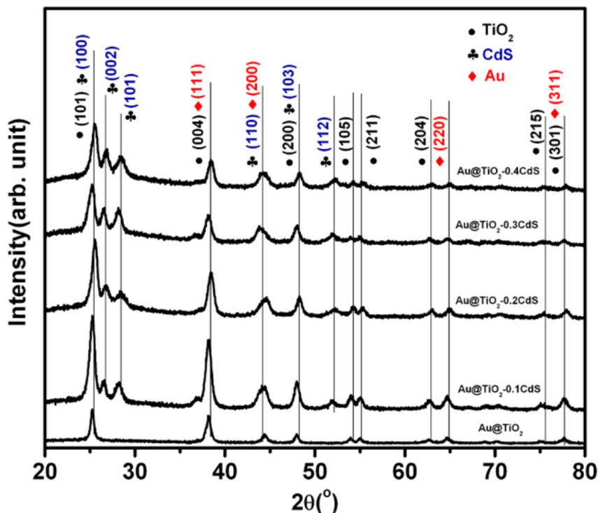
**Figure 1.** XRD patterns of various Au@TiO<sub>2</sub>-CdS nanocomposites.
