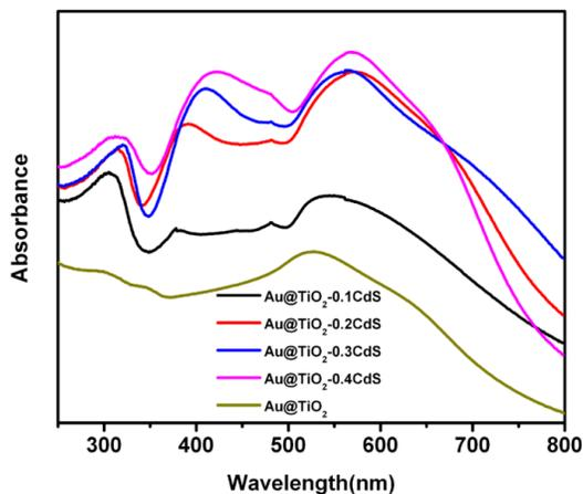
**Figure 3.** UV-vis diffuse reflectance spectra of various Au@TiO<sub>2</sub>-CdS samples.
