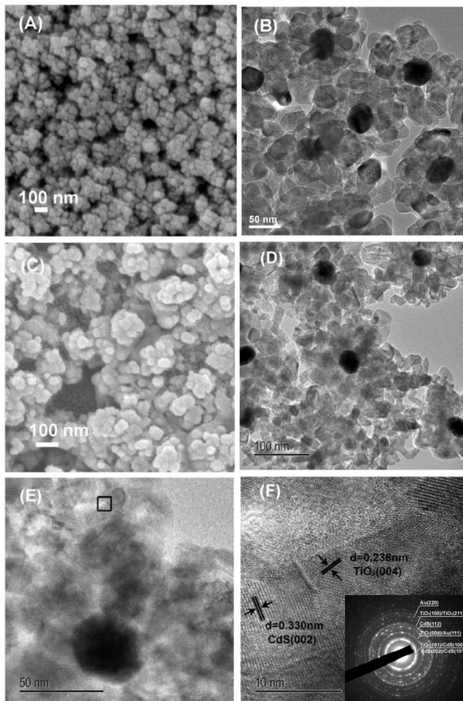
**Figure 2.** SEM and TEM images of the as-prepared Au@TiO<sub>2</sub>-CdS nanocomposites. (A) SEM image of Au@TiO<sub>2</sub>; (B) TEM image of Au@TiO<sub>2</sub>; (C) SEM image of Au@TiO<sub>2</sub>-0.2CdS; (D) and (E) TEM images of Au@TiO<sub>2</sub>-0.2CdS; (F) HRTEM image of Au@TiO<sub>2</sub>-0.2CdS. The inset of (F) is SAED patterns of Au@TiO<sub>2</sub>-0.2CdS.
