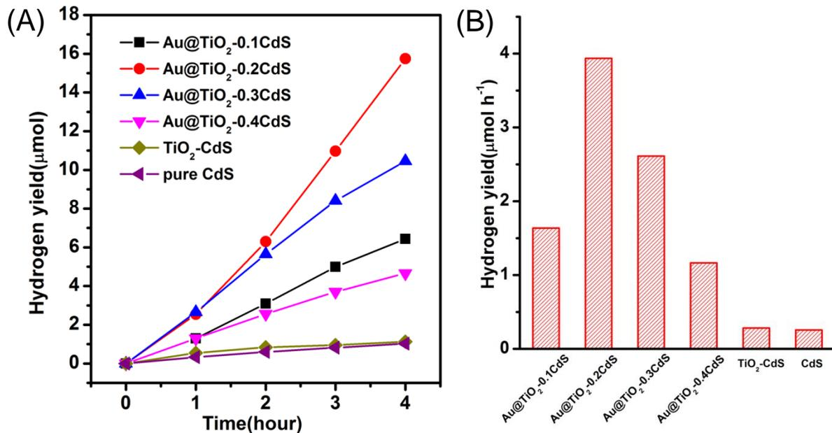
**Figure 4.** (A) Plots of photocatalytic H<sub>2</sub> evolution amount versus visible light irradiation ( $\lambda > 420$  nm) time by various samples; (B) The H<sub>2</sub> evolution rate by various samples.
