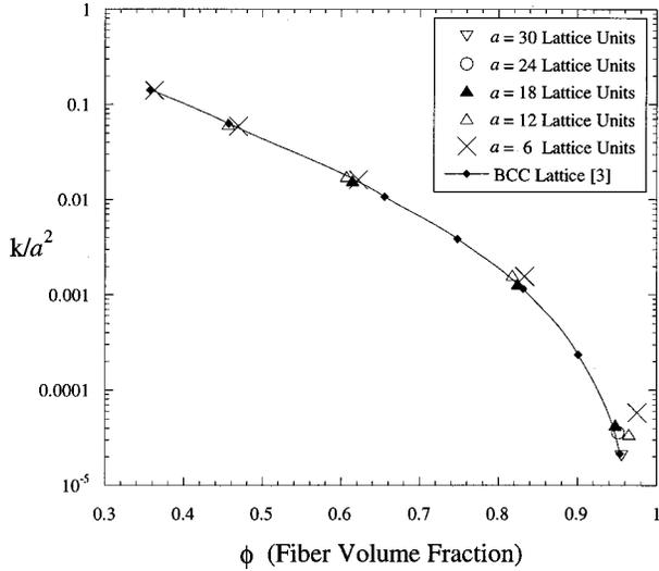
FIG. 6. Resolution study using the bcc lattice. The hydraulic permeability is calculated using the LB method for various cylinder radii  $a$  at moderate to high fiber volume fractions  $\phi > 0.35$ . The results are compared with the results of Higdon and Ford [3] for the same configuration of cylinders. The line through their data is provided to guide the eye.
