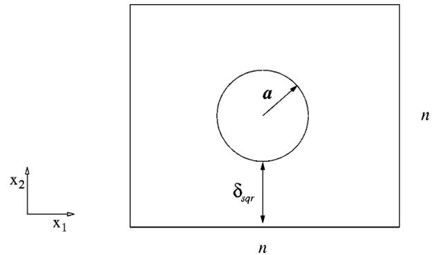
FIG. 1. Two-dimensional simulation cell for a square array of periodic cylinders. The simulation cell consists of a cylinder of radius  $a$  centered in a square cell. The simulation cell edge length is  $n$ .  $\delta_{sqr}$  is the distance from the surface of the cylinder to the edge of the cell or the half distance between periodic cylinders.
