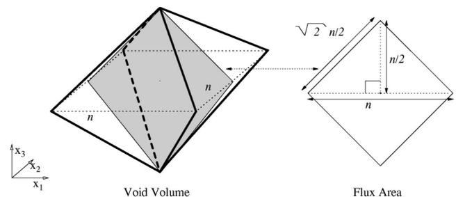
FIG. 3. Void volume formed by two adjacent bcc simulation cells. The bold lines represent the cylinders in the foreground of the system; the bold dashed lines represent the the cylinders in the background. The inscribed shaded region, a square, represents the flux area where the fluid flows. The edge length for an individual, cubic simulation cell is  $n$ .
