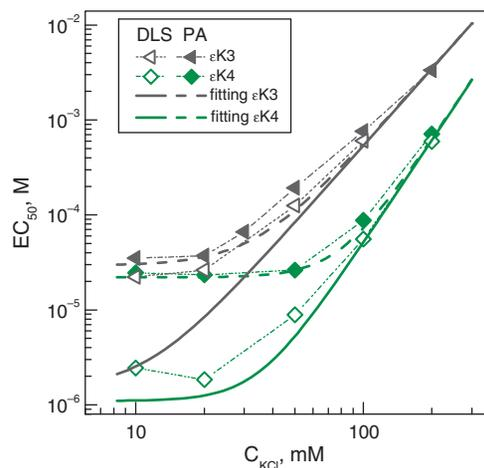
**Figure 9.** Comparison of the experimental dependencies (points with thin lines) with prediction based on Equation (3) (shown as smooth thick lines) for data on DNA condensation by the  $\epsilon$ -oligolysines  $\epsilon$ K3 and  $\epsilon$ K4. DLS and PA data are shown respectively as hollow and solid points. The parameters of Equation (3) are the same as in Figure 8A. See text and Supplementary Figure 4S and Table 4S) for more detail.
