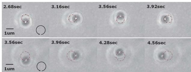
Fig. 4. (Color online) Successive frames of video recordings that show the rotation of a single gold particle trapped by PVs of  $l = 2$  (top row, Media 1) and  $l = 5$  (bottom row, Media 2). The circular arrow denotes the rotation direction, and the dashed circles show the particle's orbital trajectory.
