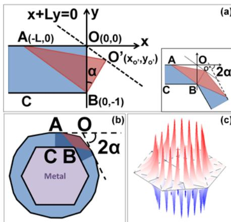
**Figure 2.** (Color online) (a) APT (from  $ABO$  to  $AB'O'$ ) for one arm of the bending adapter. (b) A transformation optics based polygonal resonator formed by multiple bending adapters. (c) The distribution of magnetic field of a transformation optics based SP hexagonal resonator.
