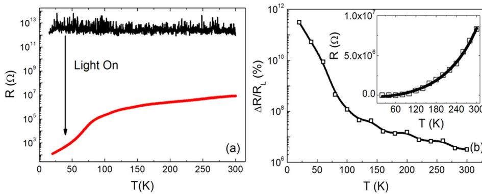
FIG. 3. (a) The temperature dependence of the resistance of bare STO single crystals with and without the light irradiations. (b) The photoinduced relative change in resistance as a function of temperature. The inset shows that resistance vs. temperature curve of STO single crystals under the light irradiation. The solid line is the best fit to the data.
