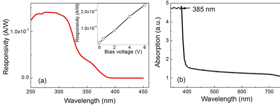
FIG. 1. (a) The normalized steady-state photoresponsivity spectra as a function of wavelength for the as-received STO single crystals. The inset is the bias dependence of the photocurrent responsivities. (b) The ultraviolet-visible absorption spectrum of STO single crystals as a function of wavelength.
