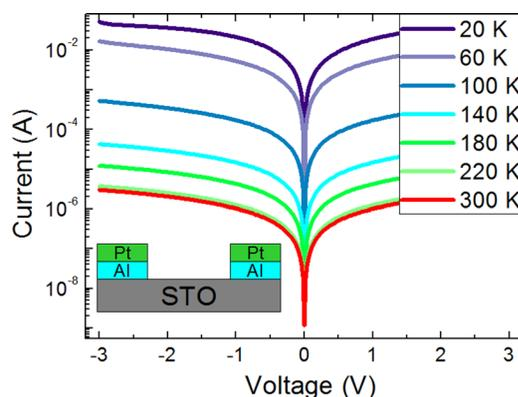
FIG. 2. The current-voltage curves in log scale of STO single crystals under the irradiation of light at different temperatures.
