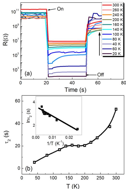
FIG. 4. (a) The time dependence of the resistance of STO single crystals under the irradiation of 365 nm. (b) The time constants as a function of temperature. The inset shows the  $\ln \tau_2$  vs.  $T^{-1}$  curve.
