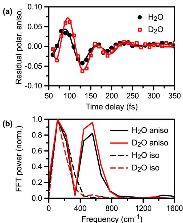
**Figure 3.** (a) The residual polarization anisotropy (symbols) reveals oscillatory features, which can be fit to a sum of two exponentially decaying cosinusoidal functions (solid lines). (b) The FFT power spectra of the residual polarization anisotropies reveal frequency components at 150 and 500 cm<sup>-1</sup> (solid lines), both of which are independent of H/D substitution. For comparison, the FFT power spectra of the isotropic signals are also shown (dashed lines).
