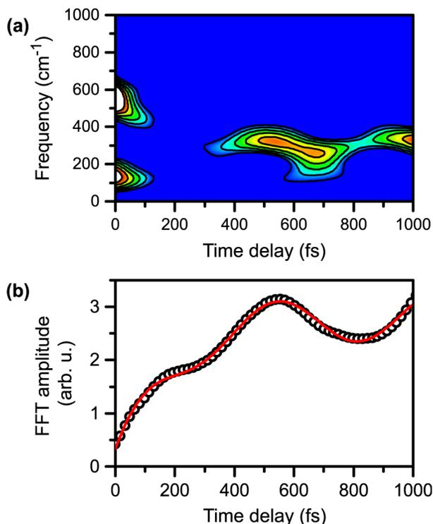
**Figure 5.** (a) The time-frequency spectrogram for the anisotropic signal shows the disappearance of the 150 and 500  $\text{cm}^{-1}$  frequency components at early times and the concomitant rise of the frequency component at 310  $\text{cm}^{-1}$ . (b) The FFT amplitude at 310  $\text{cm}^{-1}$  reveals an oscillatory rise (symbol), from which a fit to first-order kinetics (solid line) yields a lifetime of  $196 \pm 5$  fs for the aqueous  $\text{H}_2\text{O}^+$  radical cation.
