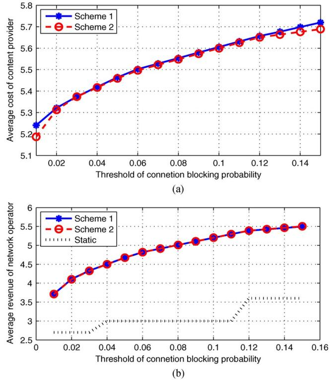
Fig. 5. (a) Average cost of content providers and (b) average revenue of network operator under different thresholds of the connection-blocking probability.
