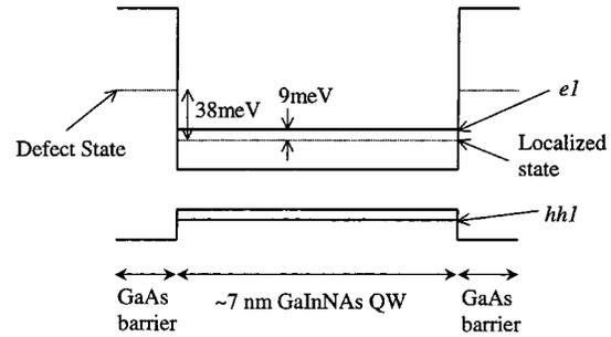
Fig. 5. Energy band diagram of PL quenching model for GaInNAs/GaAs QW.
