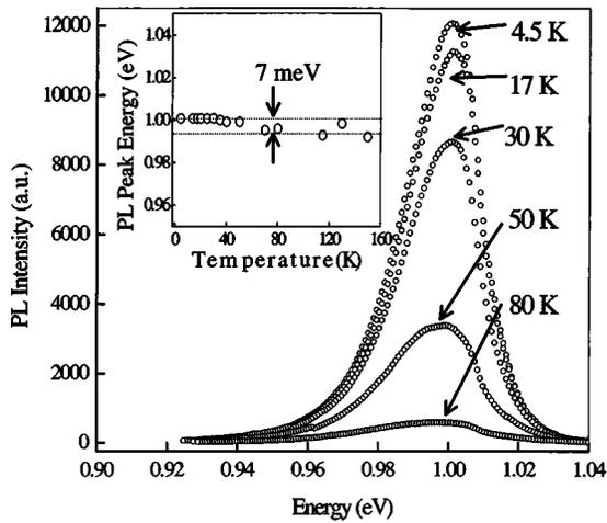
Fig. 2. Change of PL intensity in the annealed GaInNAs QW with temperature. The inset shows the change in the PL peak energy of the annealed GaInNAs QW with temperature.
