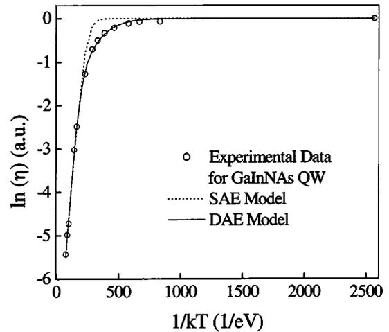
Fig. 3. Plot of PL efficiency vs inverse of temperature. The SAE model (dotted line) and DAE model (solid line) are used to fit the experimental data.
