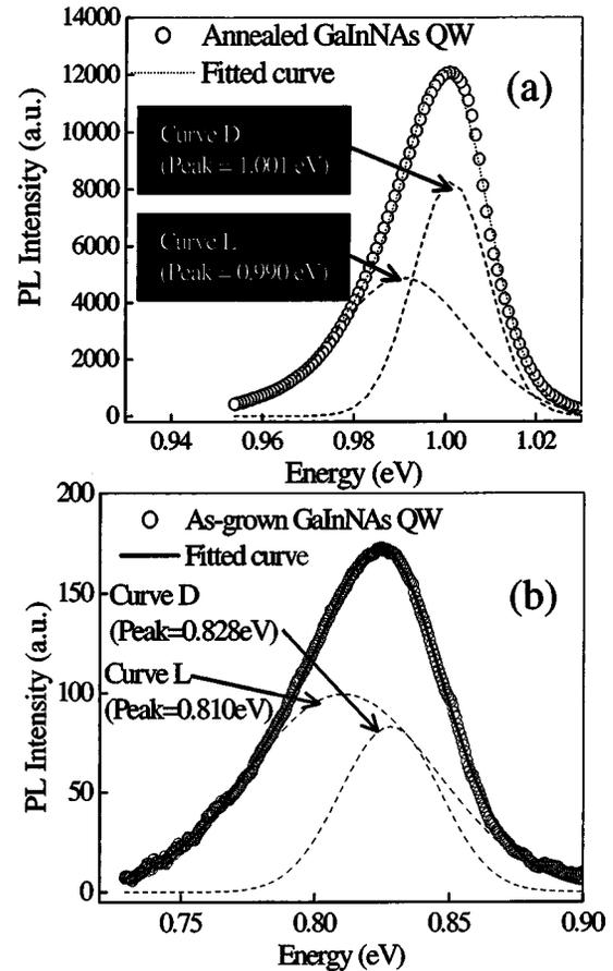
FIG. 1. 4 K PL characteristics of: (a) thermal-annealed GaInNAs/GaAs QW and (b) as-grown GaInNAs/GaAs QW. Both are fitted with two Gaussian functions.
