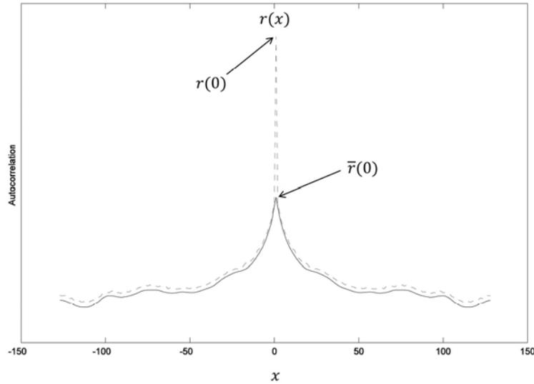
**FIGURE 1:** The autocorrelation function representation of noisy SEM image [4,5]
