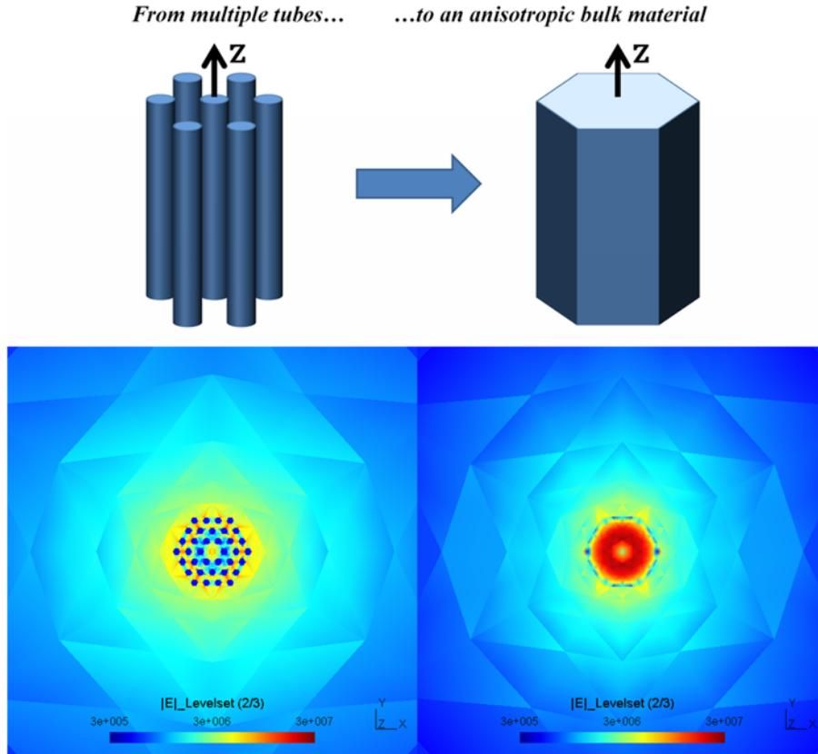
Fig. 1. Schematic illustration of the effective medium model and radial electric field distribution in a CNT monopole showing the equivalence of the hollow tube model (left) and the effective medium (right).
