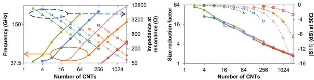
Fig. 5. Simulated characteristics of 50- $\Omega$ -fed planar SWCNT-based dipoles as a function of ( $N_{CNTs} L_{CNT}$ ). (a) Resonance frequency and input impedance. (b) Size reduction and return loss. Dipole lengths are 40 ( $\blacktriangle$ ), 80 ( $\bullet$ ), 160 (X), 320 ( $\blacklozenge$ ), and 640 ( $\blacksquare$ )  $\mu\text{m}$  with 4  $\mu\text{m}$  gap.
