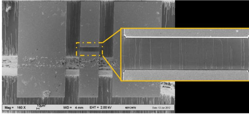
Fig. 4. Demonstration of the fabrication process by the fabrication of Au/Ti CPW gap electrodes over CVD grown CNTs.
