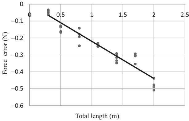
Fig. 7. Results of length effect test with  $\bar{e}$  plotted against overall length  $L$  of TSS. Each dot represents one test trial. A notable correlation can be observed between length and  $\bar{e}$  from the repeated test results.
