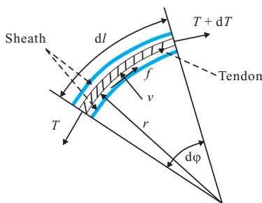
Fig. 1. (Colour online) A small segment of a tendon-sheath system.
