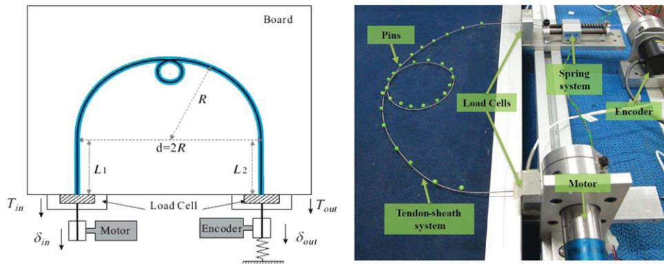
Fig. 3. (Colour online) The experimental platform with a TSS configuration in 2D. On the left is the illustration; on the right is a photo of the real experimental platform.
