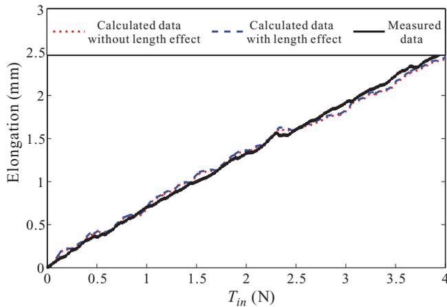
Fig. 8. (Colour online) Results of elongation test with  $L = 2$  m. Calculated data fits measured data well. However, length has a much smaller effect to elongation than to tension transmission.
