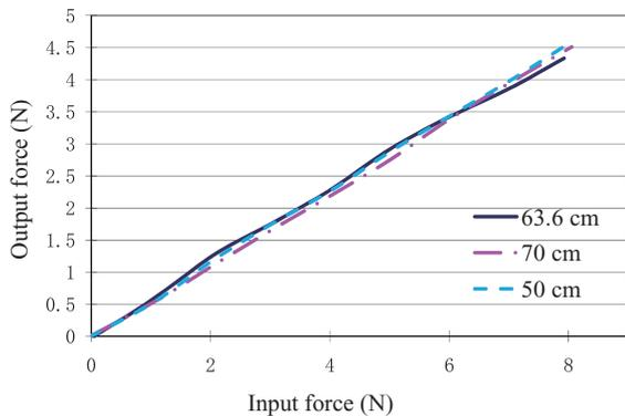
Fig. 5. (Colour online) Experimental results with  $d$  set to 50 cm, 63.6 cm, and 70 cm, with the length 1m. While curve path changes, by having the same total curve angle, the transmission ratio remains the same.
