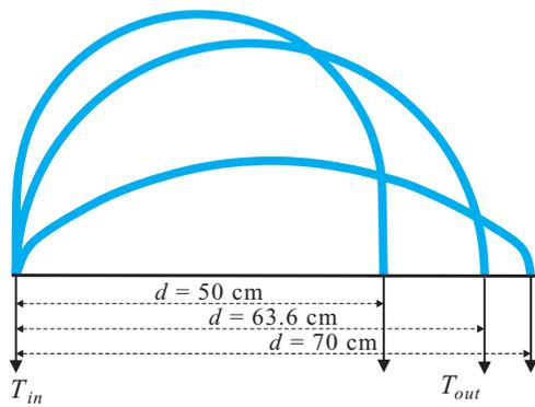
Fig. 4. (Colour online) TSS configurations with  $d$  set to 50 cm, 63.6 cm, and 70 cm.
