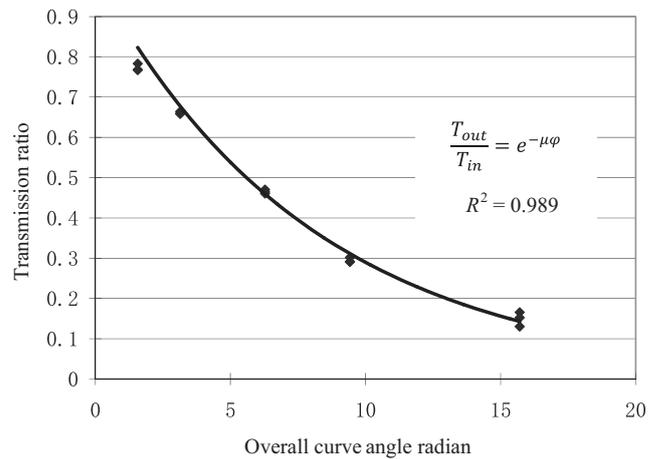
Fig. 6. Experimental results with TSS length of 1m,  $\phi$  set to  $\pi/2$ ,  $\pi$ ,  $2\pi$ ,  $3\pi$ , and  $5\pi$ . With TSS length unchanged, tension transmission ratio is an exponential function of the curve angle, with a coefficient of  $\mu = 0.124$ .
