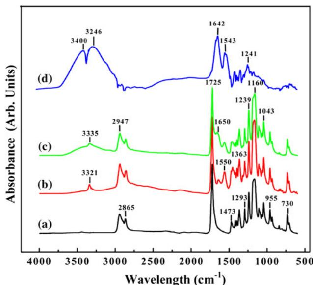
**Fig. 2** ATR-FTIR spectra of the **a** pristine PCL, **b** PCL-NH<sub>2</sub> from 1 h of aminolysis, **c** PCL-gelatin, **d** pure gelatin. The successful immobilization of gelatin was deduced from the presence of a broad band of free O-H and N-H groups (at  $3,295 \text{ cm}^{-1}$ ), amide I band (at  $1,650 \text{ cm}^{-1}$ ) and amide II band (at  $1,550 \text{ cm}^{-1}$ ) as compared to the FTIR spectrum of pure gelatin
