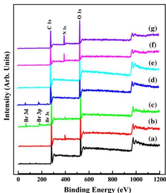
**Fig. 3** Wide scan XPS spectra of the **a** pristine PCL, **b** PCL-NH<sub>2</sub> from 1 h of aminolysis, **c** PCL-Br, **d** PCL-*g*-P(GMA)1 from 1 h of ATRP, **e** PCL-*g*-P(GMA)2 from 3 h of ATRP, **f** PCL-*g*-P(GMA)1-*c*-gelatin, and **g** PCL-*g*-P(GMA)2-*c*-gelatin surfaces
