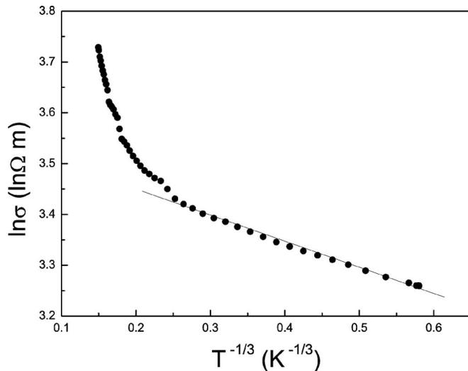
FIG. 9. Plot of  $\ln \sigma$  vs  $1/T^{1/3}$  for S1#. The solid line is the best fit of the data to formula (1) at  $T < 100$  K.
