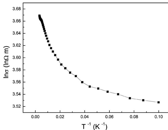
FIG. 2. Plot of  $\ln \sigma$  vs  $1/T$  for S1#.
