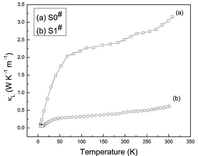
FIG. 5. Plot of lattice thermal conductivity  $\kappa_L$  vs temperature for (a) S0<sup>#</sup> and (b) S1<sup>#</sup>.
