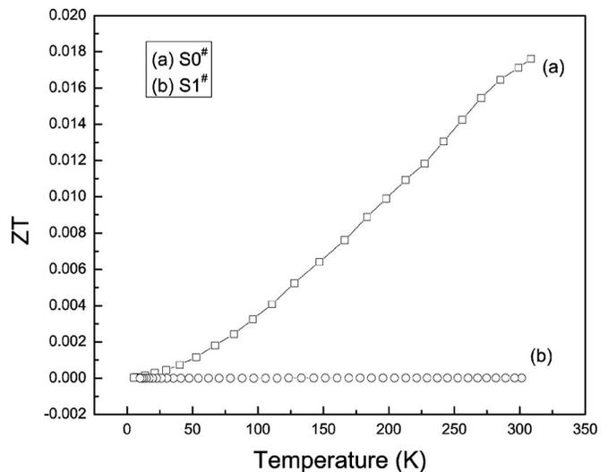
FIG. 6. Variation of  $ZT$  with temperature for (a) S0<sup>#</sup> and (b) S1<sup>#</sup>.
