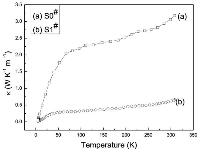
FIG. 4. Plot of thermal conductivity  $\kappa$  vs temperature for (a) S0<sup>#</sup> and (b) S1<sup>#</sup>.
