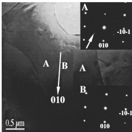
FIG. 2. 71° domain pattern viewed along  $[\bar{1}01]$ . Insets are SADPs of corresponding domains labeled A and B.  $F$  spots can be seen on the SADP of the A domain (indicated by an arrow) while no  $F$  spots are found in the SADP of the B domain.
