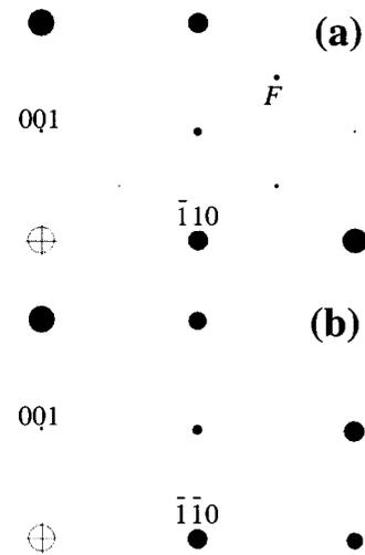
FIG. 3. Computer simulated electron diffraction pattern of PZT viewed along the  $\langle 110 \rangle$  type of zone axes. For clarity, only one quarter of the pattern is shown. The zone axis is  $[110]$  for (a) and  $[\bar{1}10]$  for (b).
