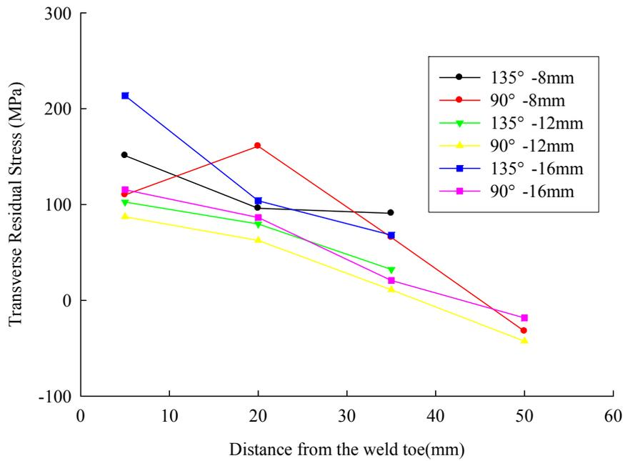
Fig. 12 Residual stresses distribution along the transverse direction (y axis) for joints welded at ambient temperature
