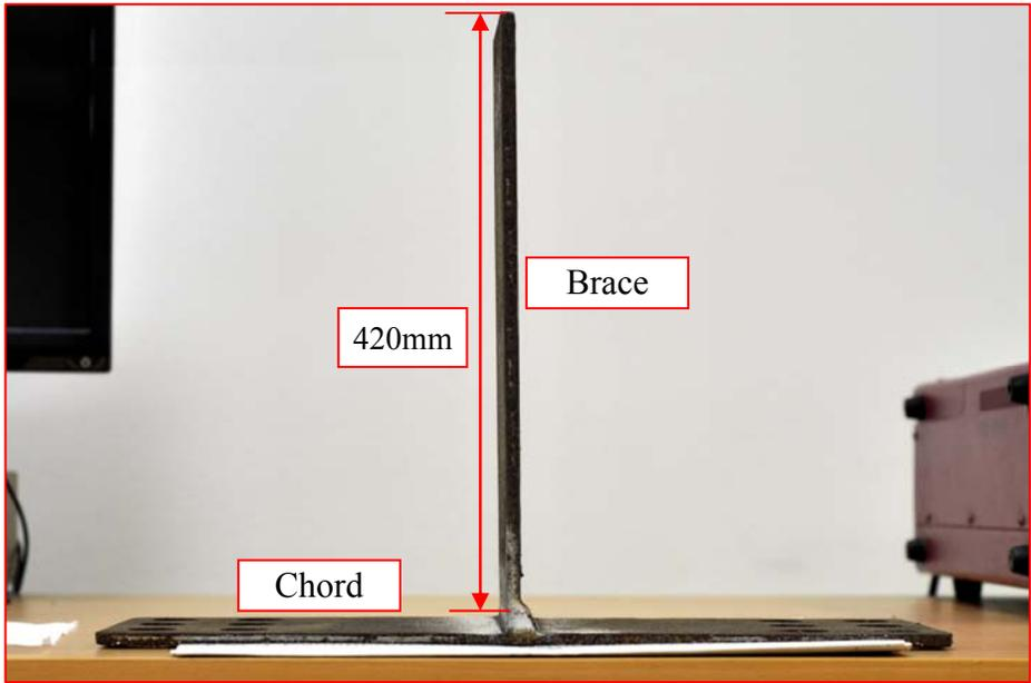
Fig. 8 A T-joint before cutting of the brace plate
