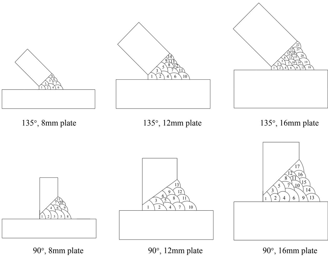
Fig. 5 The number of welding passes and welding sequences adopted for joints with different thickness and intersection angles
