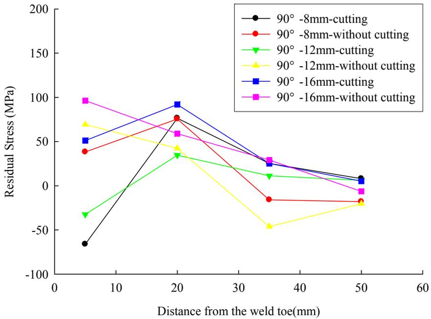
Fig. 15 Effects of brace cutting for 90° joints with preheating
