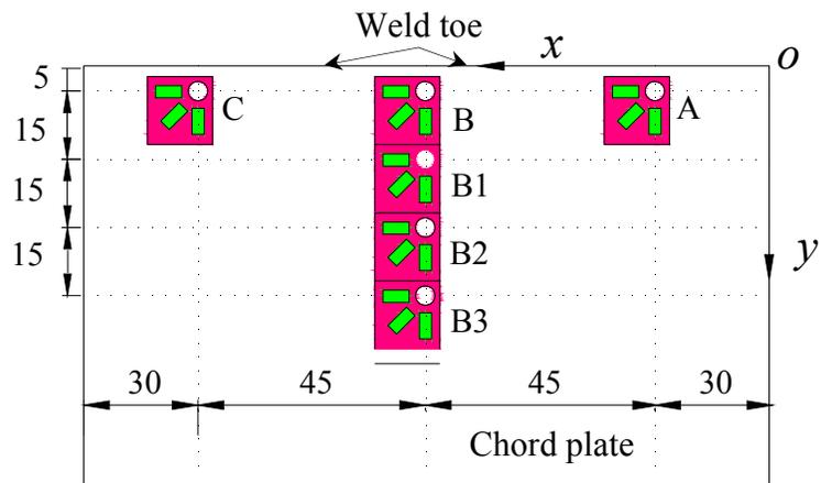
Fig. 7 Strain gauge locations on chord plate for residual stress measurement
