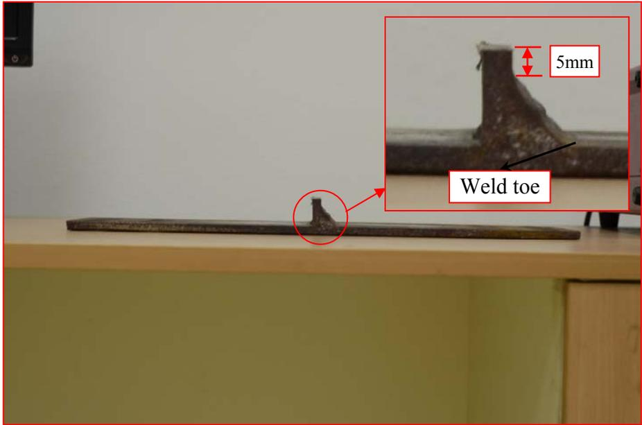
Fig. 9 A T-joint after cutting of the brace plate
