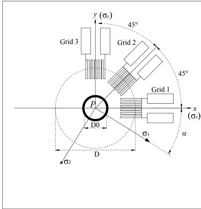
Fig. 1 Schematic diagram of strain gauge for residual stress measurement at point P
