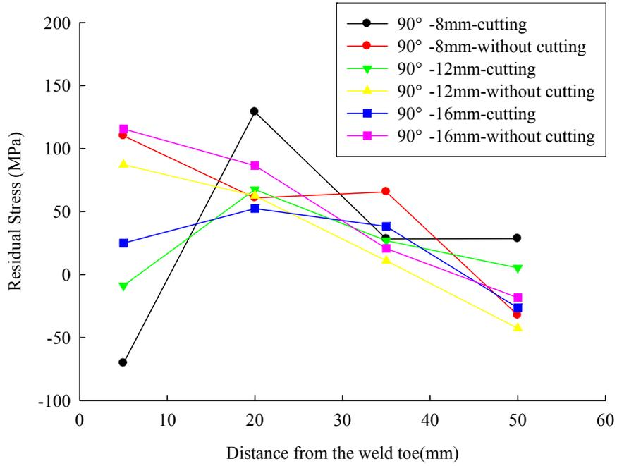
Fig. 14 Effects of brace plate cutting for 90° joints welded at ambient temperature
