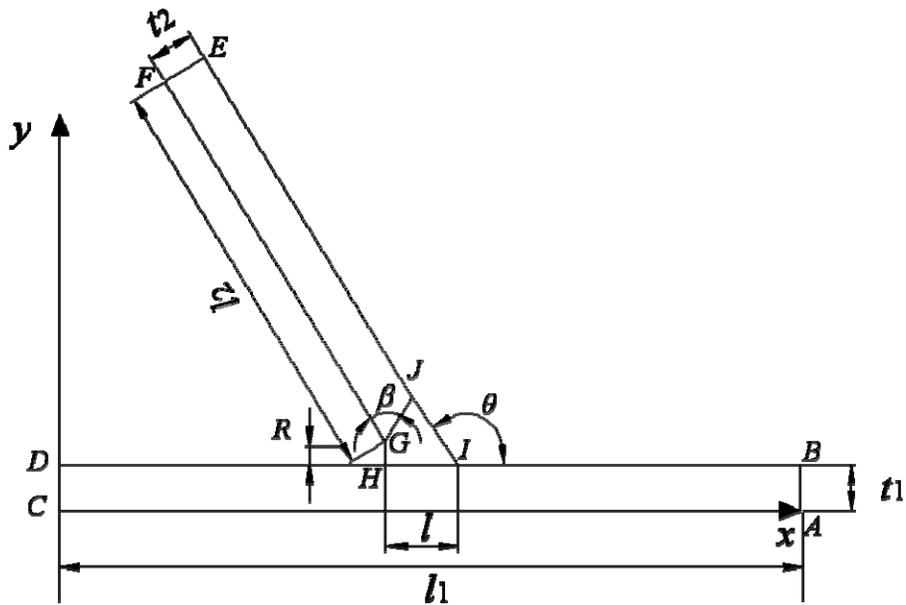
Fig. 2 Typical welding profile of plate-to-plate joint (for  $\theta=90^\circ$  and  $135^\circ$ )
