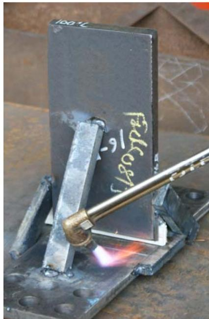
Fig. 4 The preheating process
