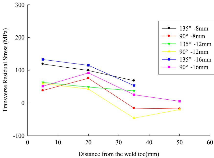
Fig. 13 Residual stresses distribution along the transverse direction (y axis) for joints with preheating
