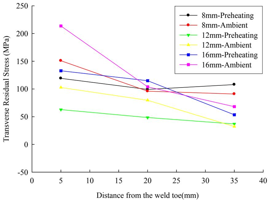
Fig. 11 Residual stresses distribution along the transverse direction (y axis, gauges B, B1 and B2) for 135° joints
