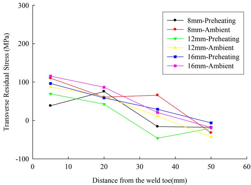
Fig. 10 Residual stresses distribution along the transverse direction (y axis, gauges B, B1, B2 and B3) for 90° joints
