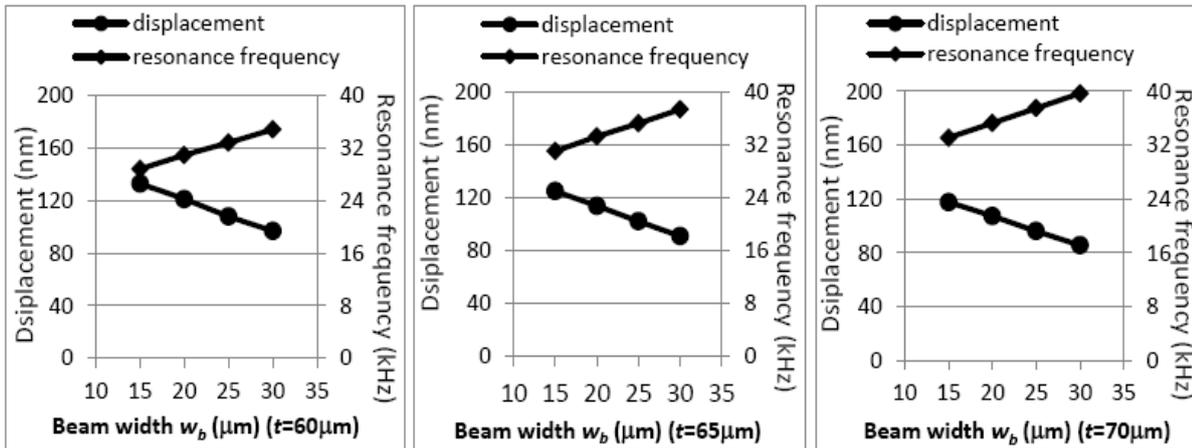
Fig. 2 Simulated displacements and frequencies varying with the beam width
