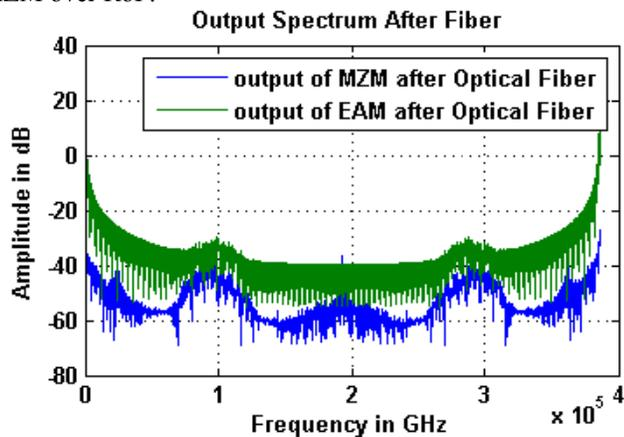
Figure 6. Output Spectrum after 1km of Fiber
