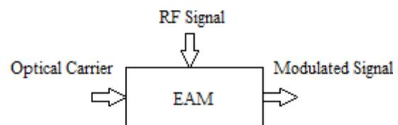
Figure 4. Electro absorption modulator
