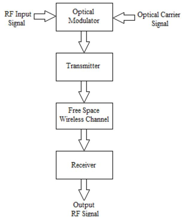
Figure 1. Block diagram of RoFSO communication system
