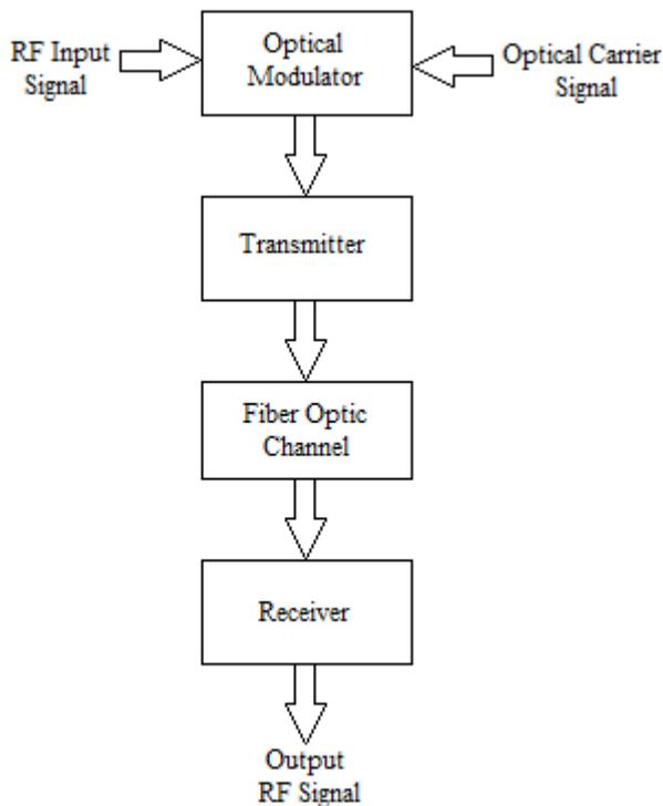
Figure 2. Block diagram of RoF communication system
