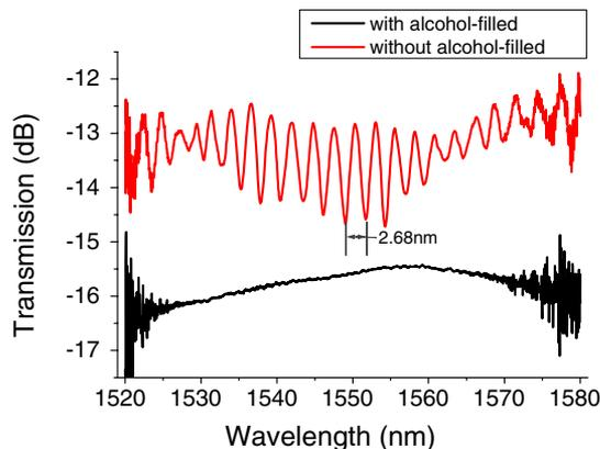
Fig. 2. Transmission spectrum with (black curve) and without (red curve) ethanol filled when no heating was applied.
