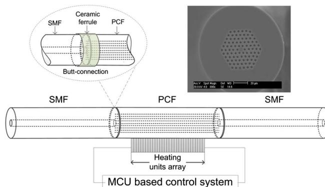
Fig. 1. Schematic diagram of the system configuration. The inset shows the cross sectional view of the PCF.
