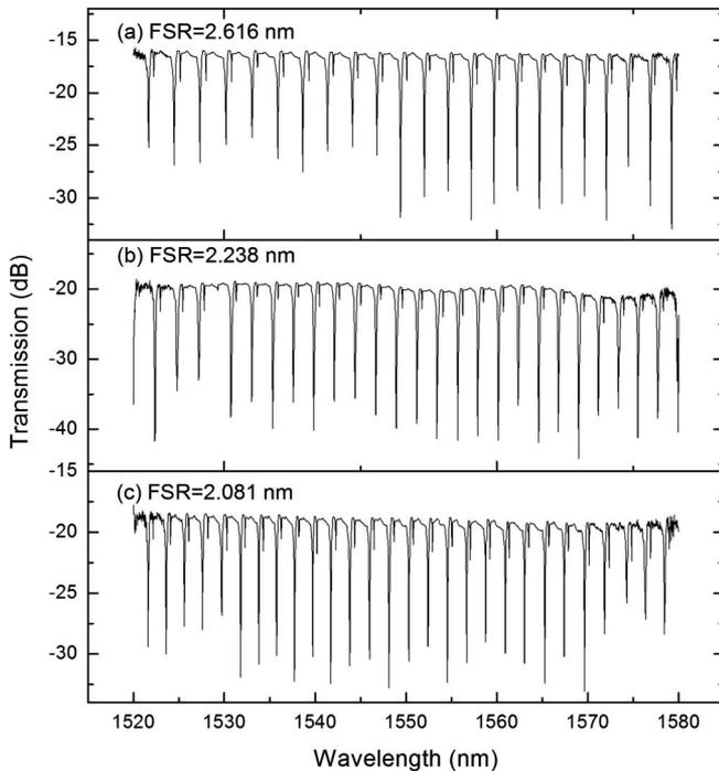
Fig. 5. Transmission spectra with different heating lengths (a) 5 mm, (b) 6.25 mm, (c) 7.5 mm, and the FSRs are 2.616 nm, 2.238 nm, and 2.081 nm, respectively.
