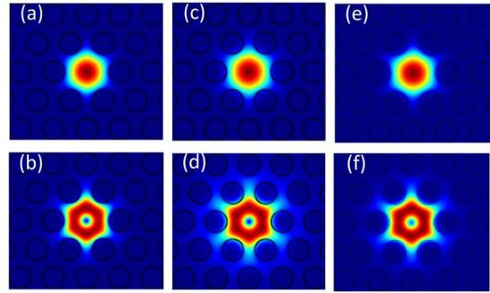
Fig. 3. Transverse mode field intensity distribution, (a), (c), and (e) HE11 mode, (b), (d), and (f) HE21 mode, when w/o ethanol filled (a) and (b), with ethanol filled but w/o heating (c) and (d), and with ethanol filled and heated (e) and (f), respectively.
