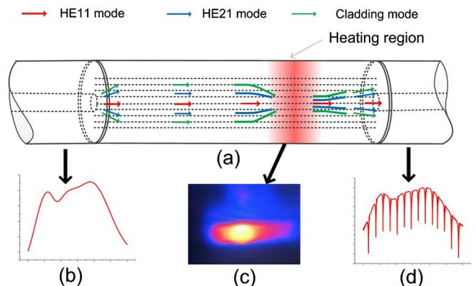
Fig. 4. (a) Schematic diagram of the thermally-induced MZI; (b) and (d) are input spectrum and output spectrum, respectively; (c) is the enlarged view of the heating region from the infrared thermal imaging camera.
