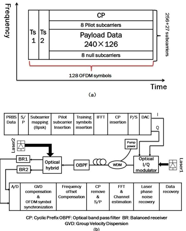
Fig. 3. (a) OFDM frame structure and (b) the schematics of the transmitter, fiber link, and receiver.
