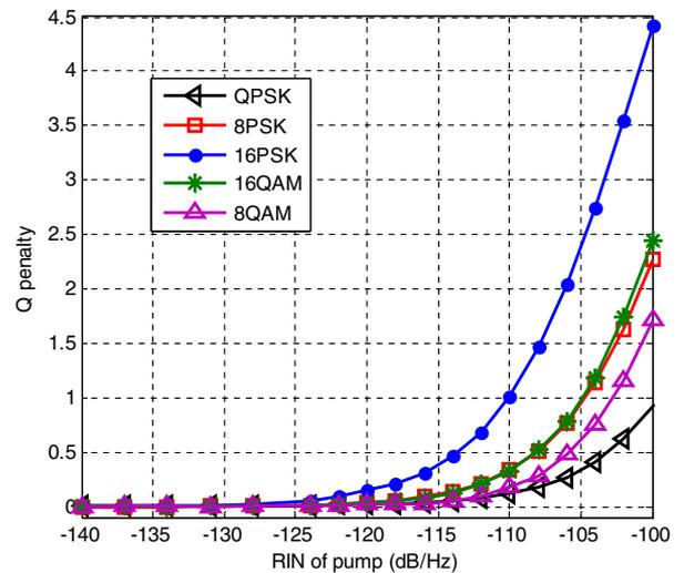
Fig. 6. Estimated  $Q$ -penalty versus pump RIN for different order PSK signals, 16QAM, and 8QAM. The walk-off parameter is 2 ps/m for all, the symbol rate is 40 GSam/s, and the linewidths of the signal laser and the LO are 100 KHz.
