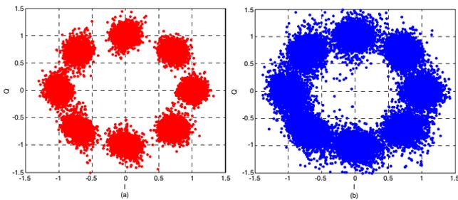
Fig. 4. Constellation of the received 8PSK-CO-OFDM signal (a) without RPN and (b) with RPN (with a variance equal to  $0.34 \text{ rad}^2$ ).
