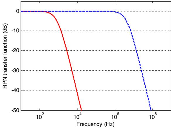
Fig. 1. RPN transfer function for Raman amplifier with walk-off is 2 ps/m, pump at 1450 nm, and signal at 1550 nm. The pump attenuation is 0.25 dB/km, the signal attenuation is 0.2 dB/km, and the length is 100 km for the co-pumping case (dotted line) and the counter-pumping case (solid line).
