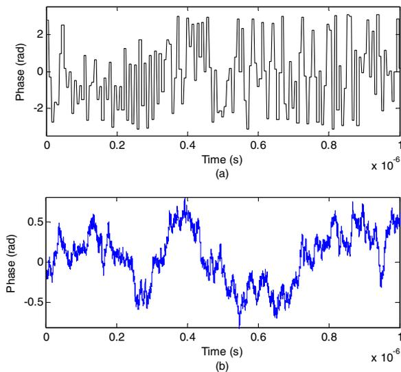
Fig. 2. Phase samples of (a) one subcarrier of the OFDM employing 8PSK and (b) the RPN in the co-pumping case (with RPN variance  $0.34 \text{ rad}^2$ ). Both are in  $1 \mu\text{s}$ .
