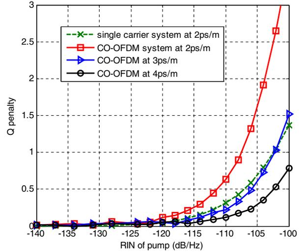
Fig. 5. Estimated  $Q$ -penalty versus pump RIN for 8PSK in the CO-OFDM system (solid line) at 2 ps/m, 3 ps/m, and 4 ps/m walk-off parameters and in a single carrier system (dashed line) at a 2 ps/m walk-off parameter. The symbol rate is 40 GSam/s, and the linewidth of the signal laser and the LO are 100 KHz.
