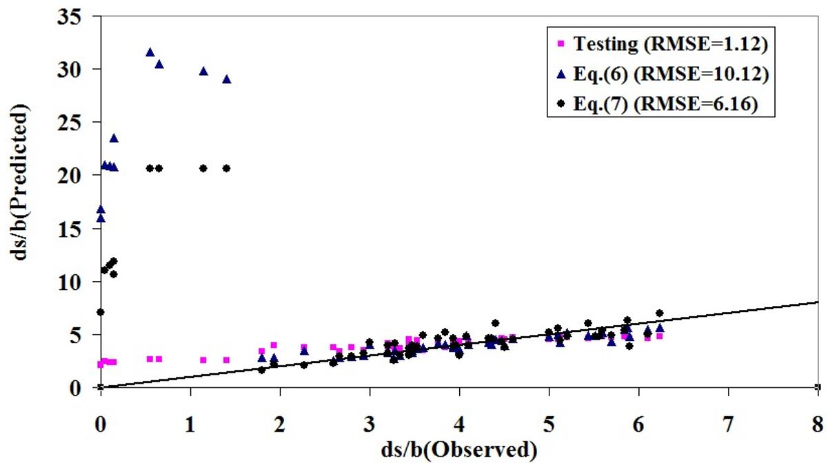
Fig. 6. Scatter plot of observed and predicted scour depth for testing stages of NF-GMDH-PSO and empirical equations.
