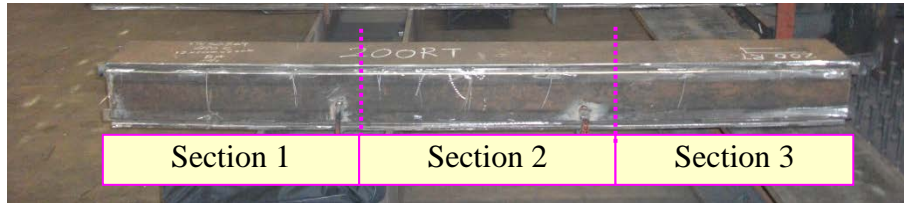
(b) Photo of fabricated box after welding
