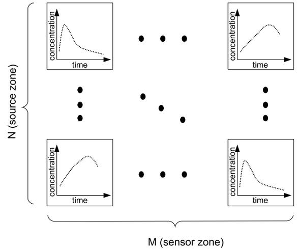
Fig. 1. Lookup table structure.  $M$  is the number of sensor zones, and  $N$  is the number of zones in the building. Each zone has at most one sensor, i.e.  $M \leq N$ .
