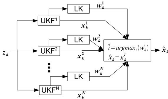
Fig. 2. The structure of the MM-UKF with  $N$  models
