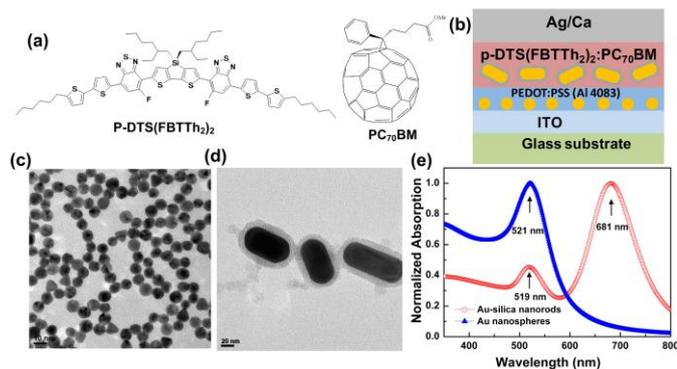
**Fig. 1** (a) Molecular structures of the p-DTS(FBTTh<sub>2</sub>)<sub>2</sub> and PC<sub>70</sub>BM, (b) device structure of the SM solar cell, (c) TEM image of Au nanospheres, (d) TEM image of Au-silica nanorods and (e) normalized UV-Vis absorption spectra of Au nanospheres in water and Au-silica nanorods in CB.
