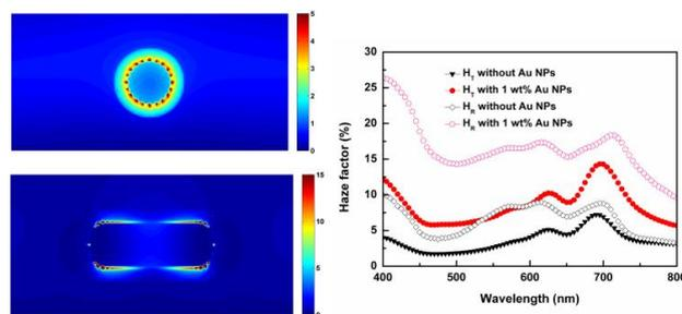
**Fig. 3** (a) Electric field distribution around Au-silica nanorods at 680 nm in front view and side view and (b) Transmission haze factor and reflection spectra for p-DTS(FBTTh<sub>2</sub>)<sub>2</sub>:PC<sub>70</sub>BM film with and without 1 wt% of Au-silica nanorods.
