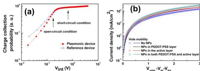
**Fig. 4** (a) Charge collection probability ( $P_C$ ) versus internal voltage ( $V_{int}$ ) characteristics of the reference device and dual NPs device and (b) the dark  $J$ - $V$  characteristics of hole-only devices with and without Au NPs.
