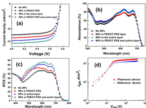
**Fig. 2** (a)  $J$ - $V$  characteristics of solar cells with and without NPs, (b) UV-Vis absorption spectra of p-DTS(FBTTh<sub>2</sub>)<sub>2</sub>:PC<sub>70</sub>BM BHJ films with and without NPs, (c) IPCE spectra of solar cells with and without NPs and (d) photocurrent density ( $J_{ph}$ ) versus internal voltage ( $V_{int}$ ) characteristics of the reference device and dual NPs device.
