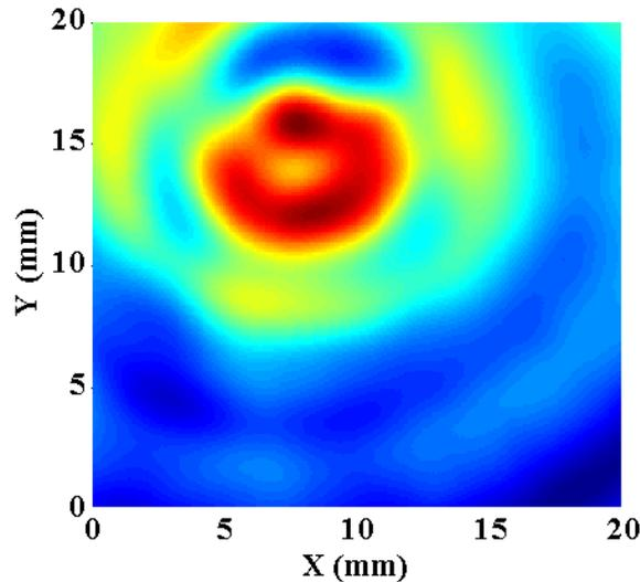
Figure 4. TA Tomography of a round metal strip.
