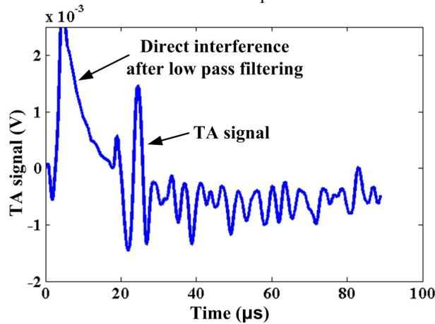
Figure 3. Detected TA signal at the first angle.
