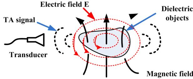
Figure 1. Schematic of magnetically mediated thermoacoustic generation
