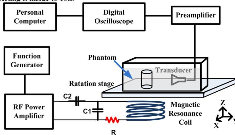
Figure 2. Experiment setup for magnetically mediated thermoacoustic signal generation and imaging
