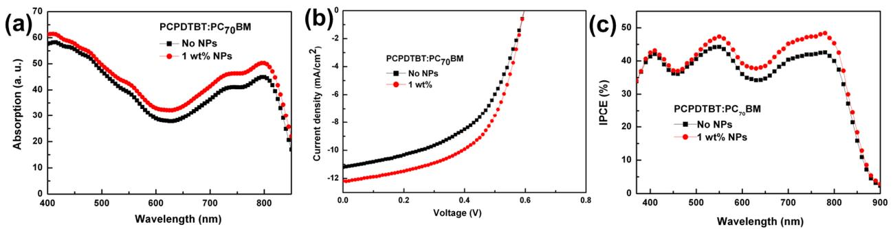
Figure 4 (a) UV-Vis absorption spectra of PCPDTBT:PC<sub>70</sub>BM BHJ films with and without NPs, (b) *J-V* characteristics of PCPDTBT:PC<sub>70</sub>BM solar cells with and without NPs and (c) IPCE spectra of PCPDTBT:PC<sub>70</sub>BM BHJ solar cells with and without NPs.
