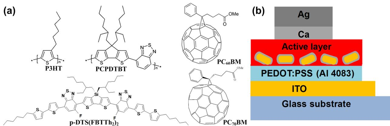
Figure 2 (a) Molecular structures of the P3HT, PCPDTBT, PC<sub>60</sub>BM, p-DTS(FBTTh<sub>2</sub>)<sub>2</sub> and PC<sub>70</sub>BM and (b) device structure of organic solar cell.
