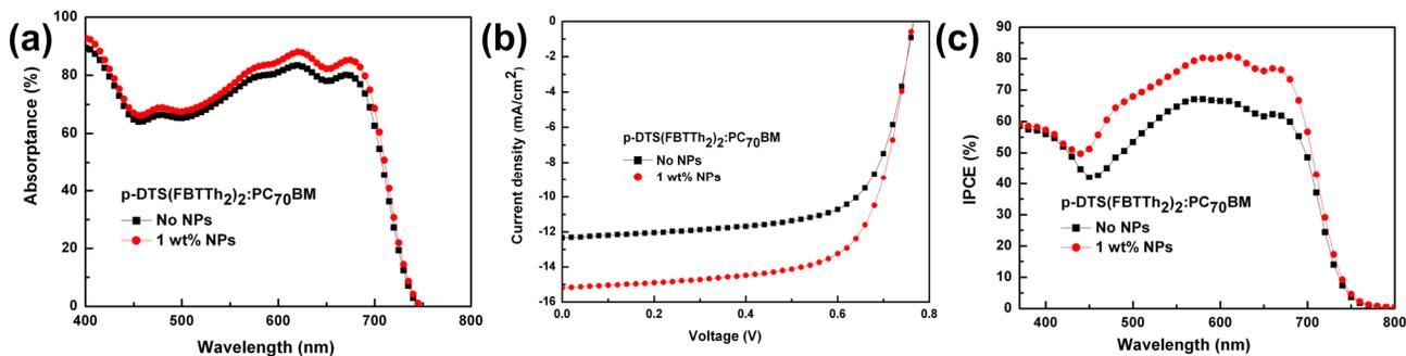
Figure 5 (a) UV-Vis absorption spectra of p-DTS(FBTTh<sub>2</sub>)<sub>2</sub>:PC<sub>70</sub>BM BJJ films with and without NPs, (b) *J-V* characteristics of p-DTS(FBTTh<sub>2</sub>)<sub>2</sub>:PC<sub>70</sub>BM solar cells with and without NPs and (c) IPCE spectra of p-DTS(FBTTh<sub>2</sub>)<sub>2</sub>:PC<sub>70</sub>BM BJJ solar cells with and without NPs.
