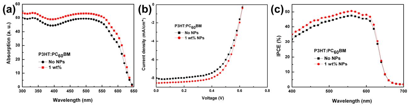
Figure 3 (a) UV-Vis absorption spectra of P3HT:PC<sub>60</sub>BM BHJ films with and without NPs, (b) *J-V* characteristics of P3HT:PC<sub>60</sub>BM solar cells with and without NPs and (c) IPCE spectra of P3HT:PC<sub>60</sub>BM solar cells with and without NPs.
