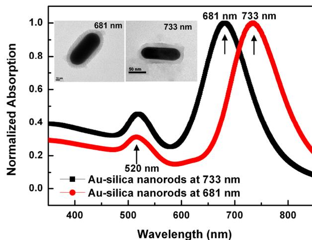
Figure 1 Normalized UV-Vis absorption spectra of two types of Au-silica nanorods with the surface plasmon resonance peaks at 681 nm and 733 nm respectively. The inset is the TEM image of corresponding Au-silica nanorods. The scale bar represents 10 nm and 50 nm respectively.
