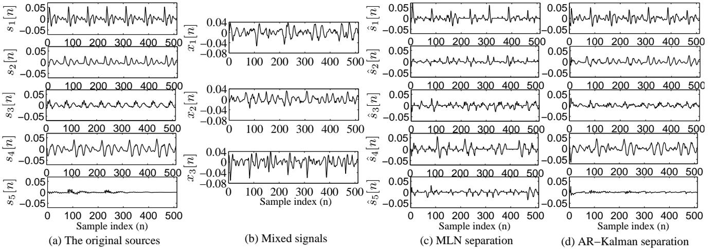
Fig. 6. Speech utterances frame of length 512 samples, their mixtures and the separated signals using MLN and AR-Kalman methods.
