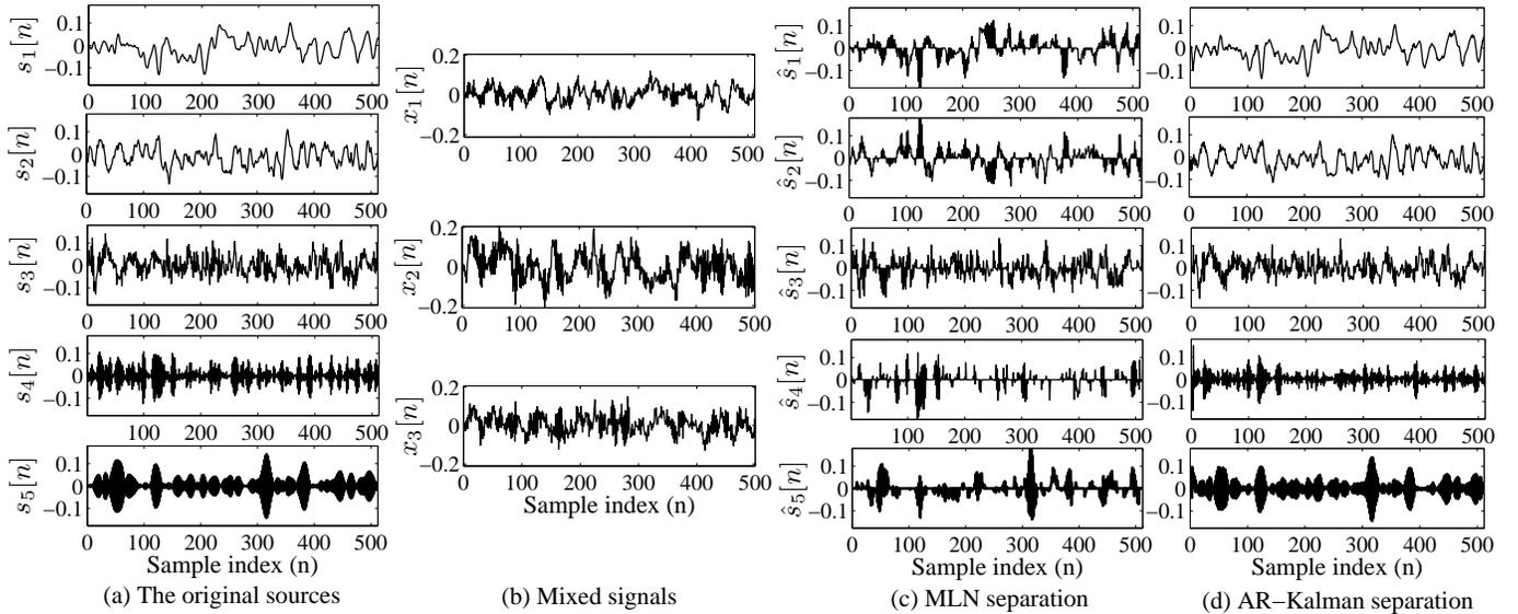
Fig. 1. Waveforms of the original signals, their mixtures and the separated signals using MLN and AR-Kalman.
