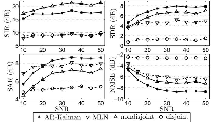
Fig. 8. Separation results of speech sources for different SNR.
