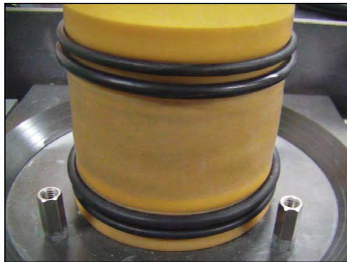
**Figure 5:** Enlarged View of Sample within Wire-Reinforced Membrane
