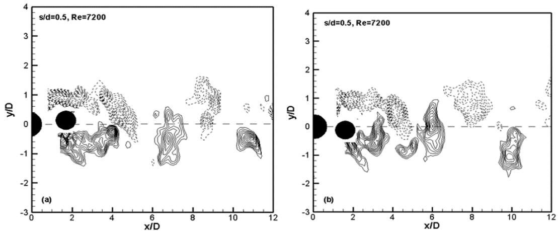
**Figure 3.** Instantaneous vorticity contours behind two tandem circular cylinders with unequal diameters ( $D/d=4/3$ ) at  $Re=7200$ ,  $s/d=0.5$ , for the downstream cylinder at its (a) highest position; (b) lowest position.
