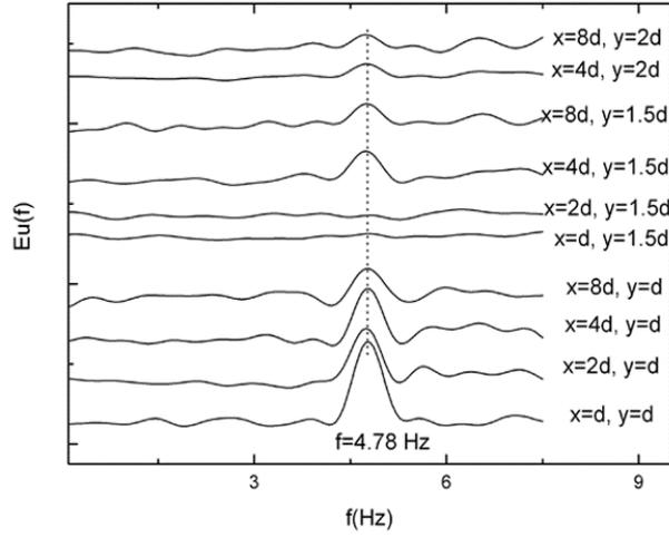
**Figure 8.** Power spectrum of velocity fluctuations at different locations behind the downstream cylinder for  $s/d=0.5$ .
