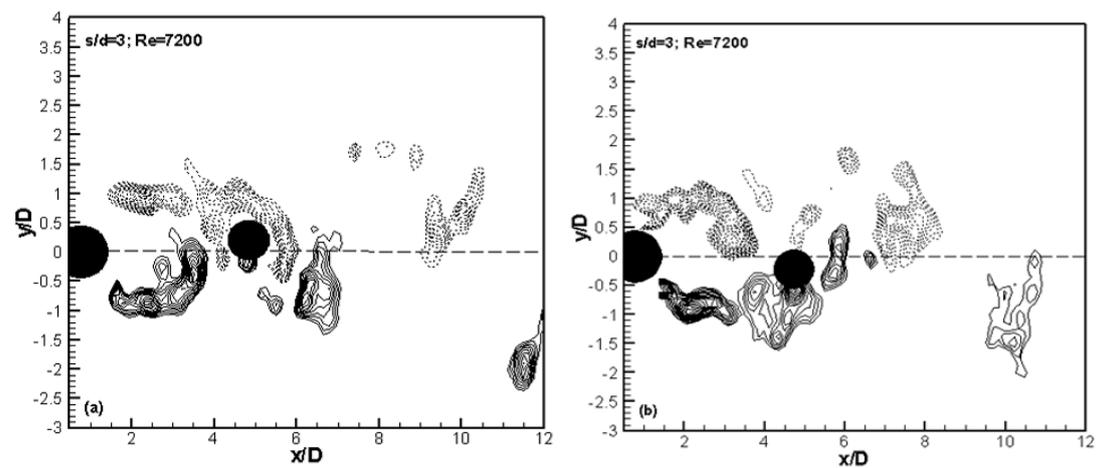
**Figure 5.** Instantaneous vorticity contours behind two tandem circular cylinders with unequal diameters ( $D/d=4/3$ ) at  $Re=7200$ ,  $s/d=3.0$ , for the downstream cylinder at its (a) highest position; (b) lowest position.
