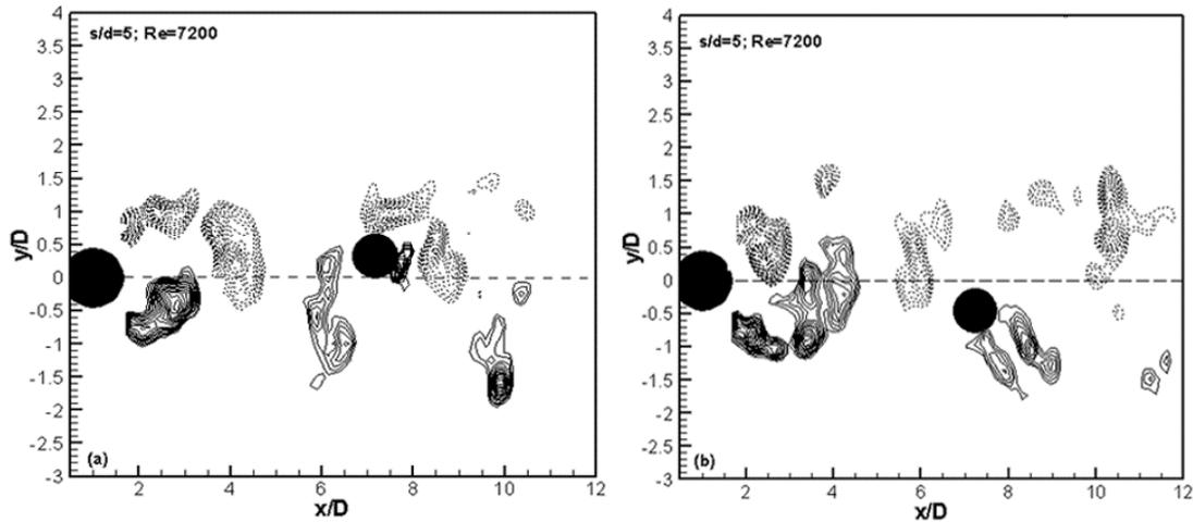
**Figure 6.** Instantaneous vorticity contours behind two tandem circular cylinders with unequal diameters ( $D/d=4/3$ ) at  $Re=7200$ ,  $s/d=5.0$ , for the downstream cylinder at its (a) highest position; (b) lowest position.
