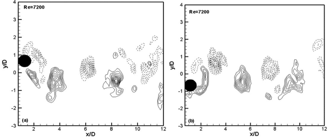
**Figure 2.** Flow visualisations employing a PIV system for a single oscillating cylinder,  $Re=7200$ , at its (a) highest position; (b) lowest position.
