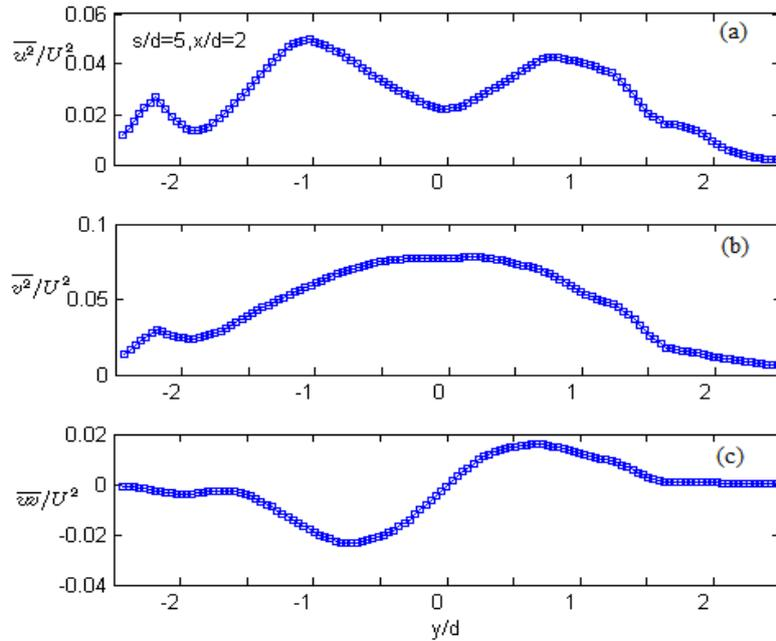
**Figure 16.** Lateral distribution of Reynolds normal stresses and shear stress at  $x/d=2.0$  behind the downstream oscillating cylinder for  $s/d=5.0$ .
