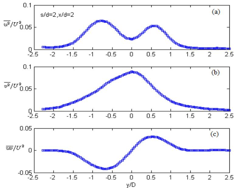
**Figure 14.** Lateral distribution of Reynolds normal stresses and shear stress at  $x/d=2.0$  behind the downstream oscillating cylinder for  $s/d=2.0$ .
