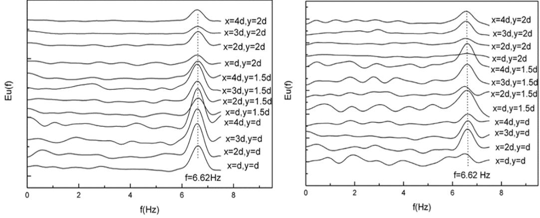
**Figure 11.** Power spectrum of velocity fluctuations at different locations behind the downstream cylinder for  $s/d=5.0$ , (a) between the cylinders; (b) behind the downstream cylinder.
