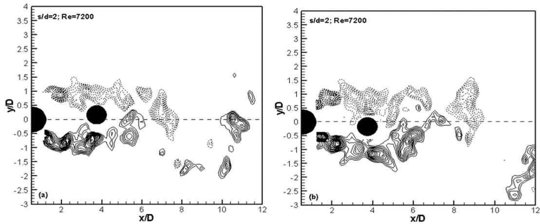
**Figure 4.** Instantaneous vorticity contours behind two tandem circular cylinders with unequal diameters ( $D/d=4/3$ ) at  $Re=7200$ ,  $s/d=2.0$ , for the downstream cylinder at its (a) highest position; (b) lowest position.
