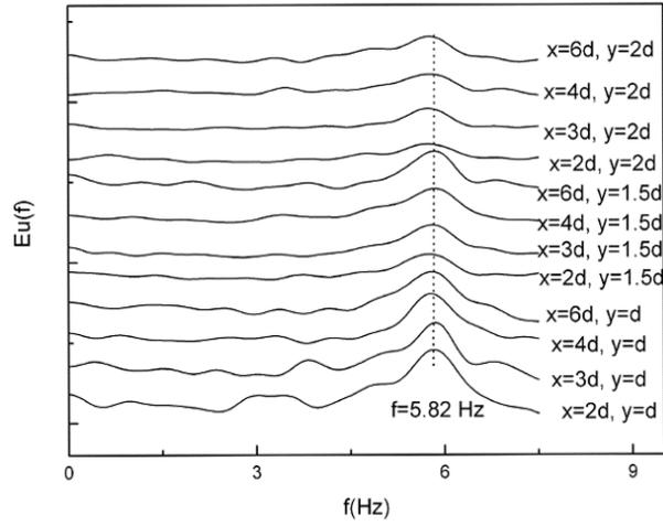
**Figure 9.** Power spectrum of velocity fluctuations at different locations behind the downstream cylinder for  $s/d=2.0$ .
