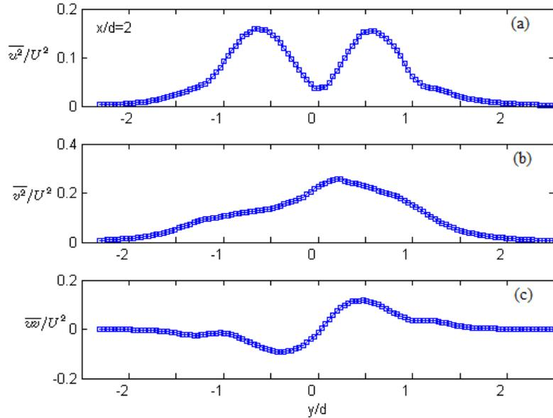
**Figure 12.** Lateral distribution of Reynolds normal stresses and shear stress at  $x/d=2.0$  for a single oscillating cylinder.
