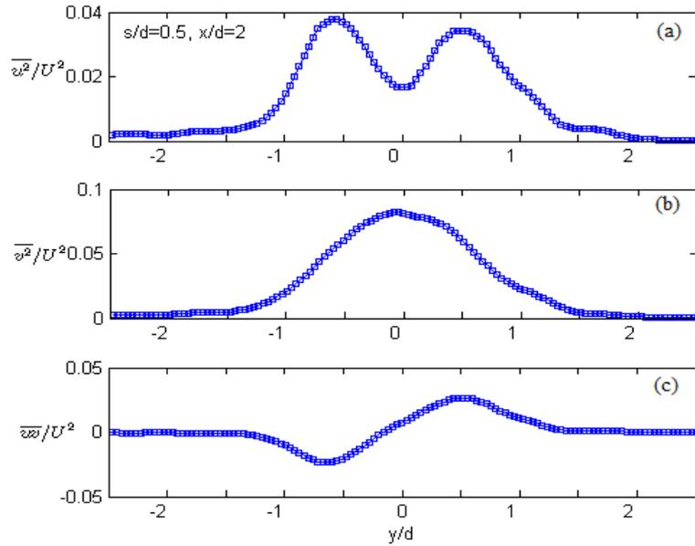
**Figure 13.** Lateral distribution of Reynolds normal stresses and shear stress at  $x/d=2.0$  behind the downstream oscillating cylinder for  $s/d=0.5$ .
