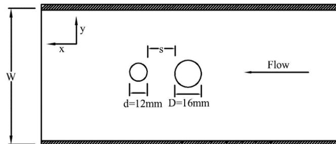
**Figure 1.** Schematic of the experimental setup, top view.
