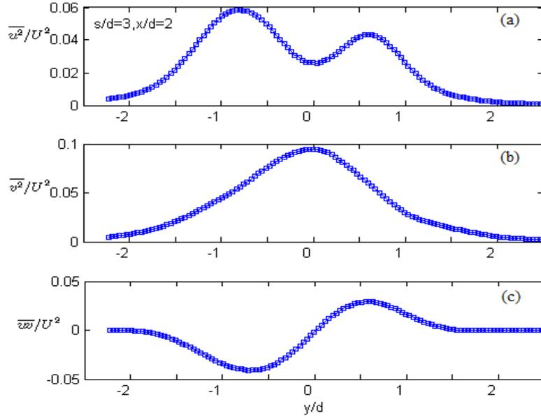
**Figure 15.** Lateral distribution of Reynolds normal stresses and shear stress at  $x/d=2.0$  behind the downstream oscillating cylinder for  $s/d=3.0$ .
