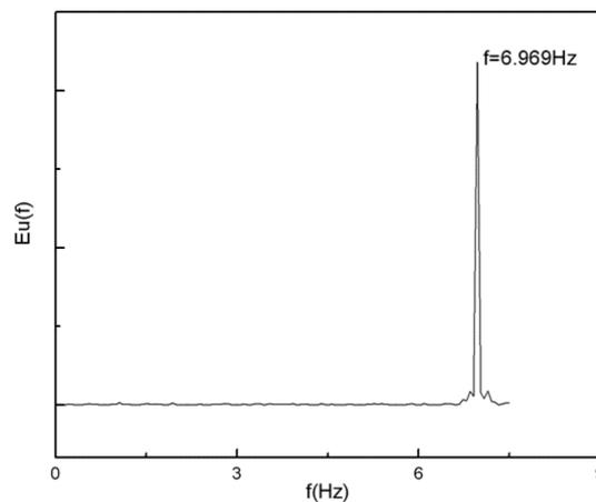
**Figure 7.** Power spectrum of velocity fluctuations behind a single oscillating cylinder.
