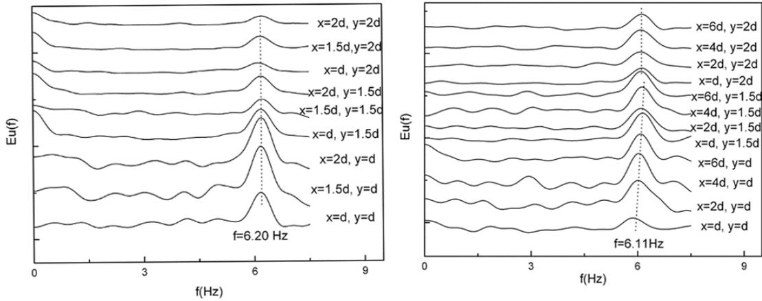
**Figure 10.** Power spectrum of velocity fluctuations at different locations behind the downstream cylinder for  $s/d=3.0$ . (a) between the cylinders; (b) behind the downstream cylinder.
