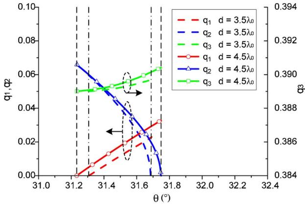
Fig. 3.  $q_m$  ( $m = 1, 2, 3$ ) as a function of  $\theta$  when  $d = 3.5\lambda_0$  and  $d = 4.5\lambda_0$  ( $\epsilon_A = 1.569^2$ ,  $\epsilon_{or} = 1.520^2$ , and  $\epsilon_{ex} = 1.725^2$ ). The black dashed-dotted/dashed lines represent the boundary values of the angular existence domain for  $d = 3.5\lambda_0/4.5\lambda_0$ , respectively.
