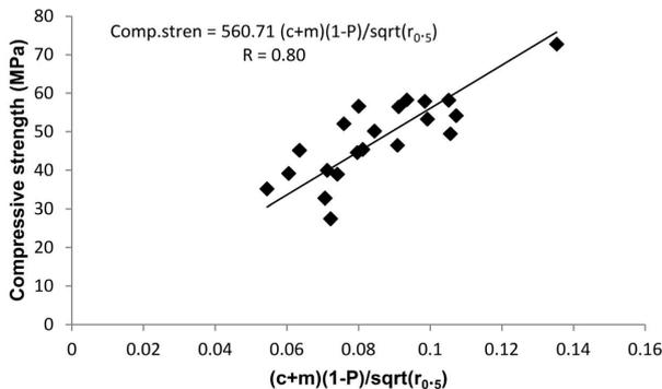
Fig.5 Compressive strength versus (c+m)(1-P)/sqrt(r<sub>0.5</sub>) plot for concrete.
