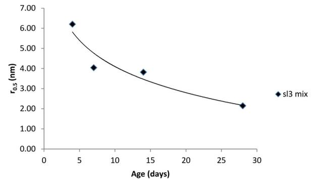
Fig.3  $r_{0.5}$  versus curing age for sl3 mix with w/c ratio 0.5.
