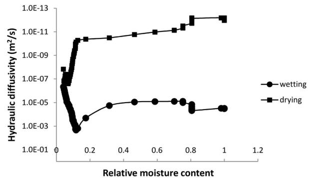
Fig.6 Hydraulic diffusivity against relative moisture content curve for sf3 mix.
