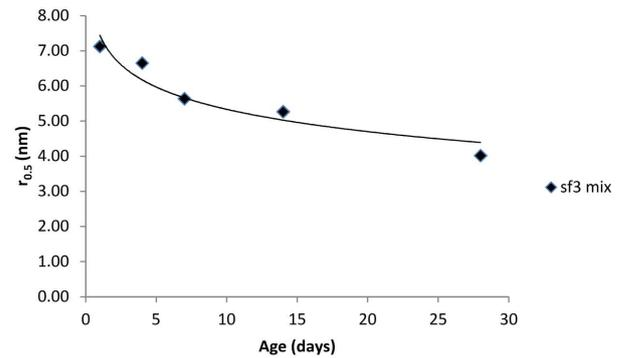
Fig.2  $r_{0.5}$  versus curing age for sf3 mix with w/c ratio 0.5.
