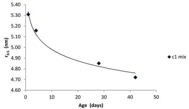
Fig.1  $r_{0.5}$  versus curing age for c1 mix with w/c ratio 0.5.
