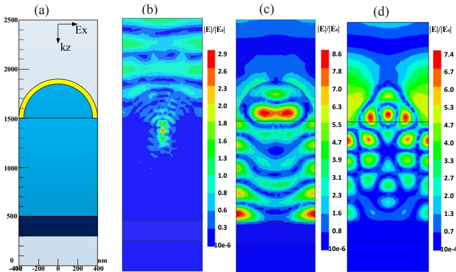
Fig. 4. Normalised electric fields across the cell structure. (a) Unit cell of the nanodome structure, (b) electric field distributions with incident light  $E_f = 2.48$  eV in the  $E_x$  direction, (c) electric field distributions with incident light  $E_f = 1.24$  eV in the  $E_x$  direction and (d) in the  $E_y$  direction.
