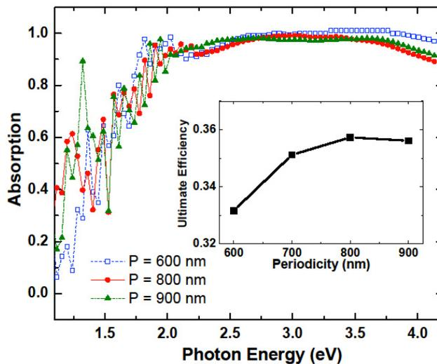
Fig. 2. Absorption spectra of nanodome structure solar cell. The inset shows the ultimate efficiency at different structure periodicity P.
