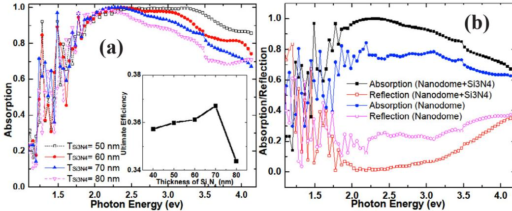
Fig. 3. (a) Absorption spectra of nanodome structure with different Si<sub>3</sub>N<sub>4</sub> thickness. The inset shows the ultimate efficiency at different Si<sub>3</sub>N<sub>4</sub> thickness. (b) Absorption and reflection spectra of nanodome structure with/without the Si<sub>3</sub>N<sub>4</sub> layer.
