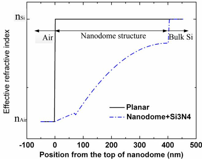
Fig. 5. The effective refractive indices of the nanodome structure as a function of depth measured from the top of the nanodome.
