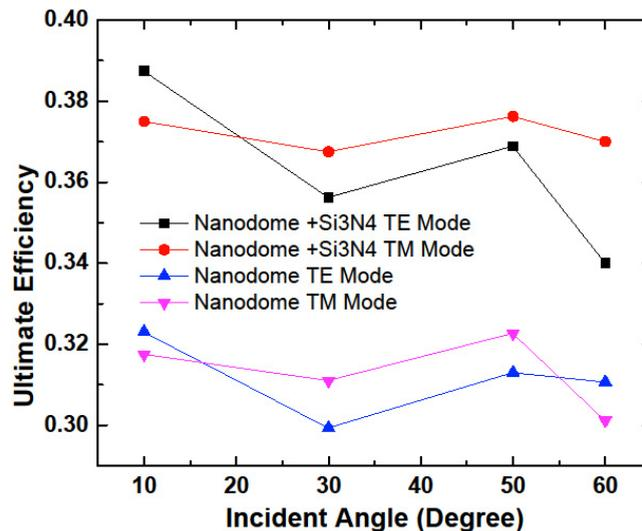
Fig. 6. Ultimate efficiency of the nanodome thin film solar cell structures with both TE and TM polarisation.
